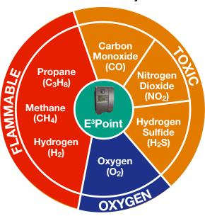
E³Point's standalone, dual-gas configuration monitors two gases simultaneously and cost effectively, in any of the following combinations: toxic-toxic, toxic-combustible, oxygen-toxic, or oxygen-combustible.
