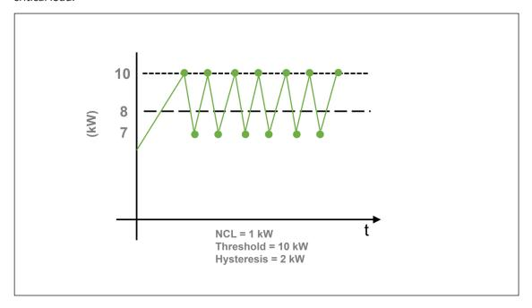
In this case, switching off the 3kW non-critical load results in the power falling below the threshold + hysteresis. This condition will result in the 3kW non-critical load switching back on again, which exceeds the 10kW threshold. The result is an infinite on/off cycling of this non-critical load. To correct this problem you must increase the hysteresis setting to a value greater than 3kW in order to prevent this infinite cycling condition.
