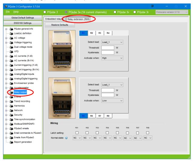
For each relay (R1 through R8), define the circuit of interest, then set the threshold, hysteresis, and threshold polarity (over-threshold or under-threshold).
