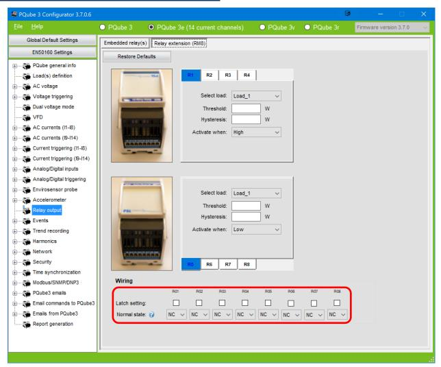
Enabling the latch setting forces the state of the relay to persist through a PQube 3 system reboot. When the latch setting is disabled, it will switch to its non-normal state (i.e., alarm state) during the reboot process. Upon completion of the PQube 3 reboot, it will return to its normal state unless the circuit load exceeds the threshold.
