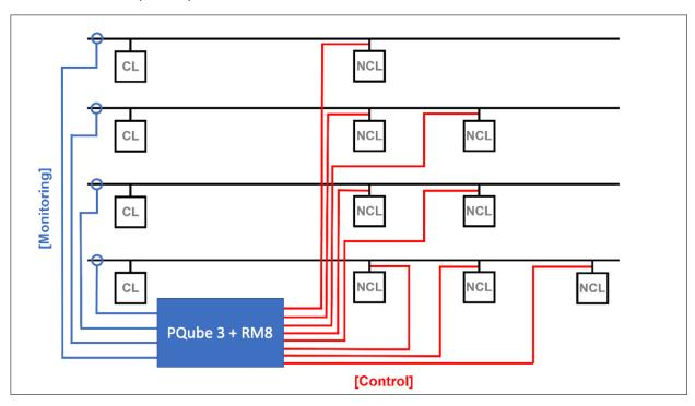
Typical use case: Monitor branch circuits powering critical loads (CL). Upon a rise above preset power thresholds or other alarm conditions, the RM8 Module turns off non-critical loads (NCL).
