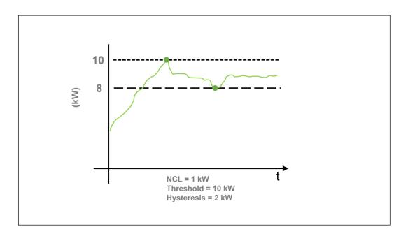
For circuit #1 an over-threshold (i.e., activates when high) of 10kW and a hysteresis of 2kW is shown.
