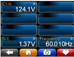
**Voltage and Frequency:** These are line-to-line, line-to-neutral, and neutral-to-earth true-RMS voltmeters. Different meters will show on these screens, depending on your power configuration. (For example, if the power configuration is “delta”, there will not be any L-N meters, because there is no neutral conductor.) If you have set a potential transformer ratio in your **Setup.ini** file, the values will reflect this ratio.
