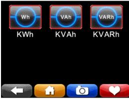
**Energy:** These three meters show the total energy, apparent energy, and reactive energy. The energy accumulators can be reset by pressing the reset numbers.
