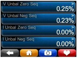
**Unbalance:** These meters show the voltage unbalance and the current unbalance. You choose in your **Setup.ini** file whether your PQube calculates unbalance using the ANSI C84.1 method, or the IEC method, or the GB method.
