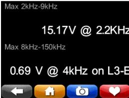
**2-150kHz:** Use this screen to view the conducted emissions in the 2-150kHz range. Useful for monitoring noise due to interference sources including solar inverters.
