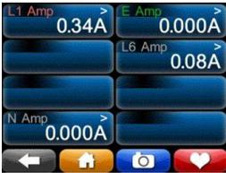
**Current:** These meters show the true-RMS current. If you have set a current transformer ratio in your **Setup.ini** file, then these meters will use that ratio, so these meters will sometimes show their values in kilo-amps or even mega-amps. Different meters will show on this screen, depending on your power configuration. (For example, if the power configuration is “delta”, this screen will not show a neutral current meter, because there is no neutral conductor in delta power.)
