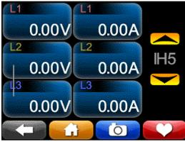
**Interharmonics:** Use this screen to view every interharmonic up to the 50<sup>th</sup> for both voltage and current. Select one harmonic at a time. The selected interharmonic applies to all channels. (Harmonic values up to the 63<sup>rd</sup> are recorded in your PQube 3's CSV files.)
