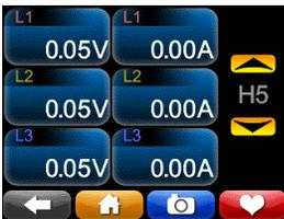
**Harmonics:** Use this screen to view every harmonic up to the 50<sup>th</sup> for both voltage and current. Select one harmonic at a time. The selected harmonic applies to all channels. (Harmonic values up to the 63<sup>rd</sup> are recorded in your PQube 3's CSV files.)
