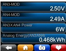
**Analog Channels:** The Analog meters show the RMS voltage (equivalent to DC voltage for DC signals). You can view the Analog-to-Earth channels (common mode) and the Analog-to-Analog channels (differential mode).
