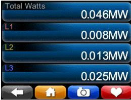
**Power:** These are the true power, apparent power, and reactive power readings, and they correctly handle harmonics (distorted voltages and distorted currents). If you have set a current transformer ratio and/or potential transformer ratio in your **Setup.ini** file, then these meters will reflect those ratios.
