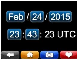
**Date/time:** You can change the time and day unless you are configured to synchronize on SNTP or NTP, or your PQube 3 is connected to GPS.
