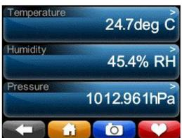
**Environmental Meters:** If you have ENV2 environmental probes, you can view your temperature, humidity, barometric pressure, acceleration, thermocouple input, and solar irradiance input here.
