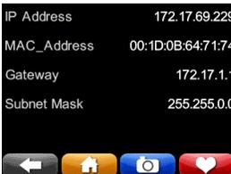
**Network:** Your PQube 3's IP address and MAC address can be found on this screen. This is useful if you have a dynamic IP address. It is also useful for troubleshooting connectivity issues. An external cable must be plugged in.
