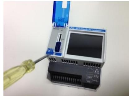
To remove and replace the battery, insert a small flat-head screwdriver to pry up the label near the USB port and microSD card slot. Remove the old battery and install the new one. It is not possible to install the battery with the wrong polarity.
