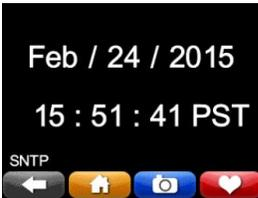
If you have enabled SNTP or NTP in your **Setup.ini** file, your PQube 3 will synchronize to UTC time, then it applies the offset from UTC as specified in your Setup file so that all measurements are time tagged with local time (in this example Pacific Time PST).
