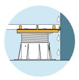
The U-Edge creates a space between the paving slab and wall keeping an even gap and enabling water flow which protects the terrace in the case of heavy rainfall, snow etc.
