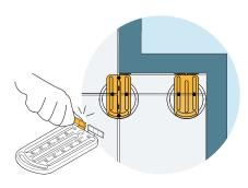
It is also possible to remove the tile retainers to adapt the U-Edge to work with all types of terrace layout.
