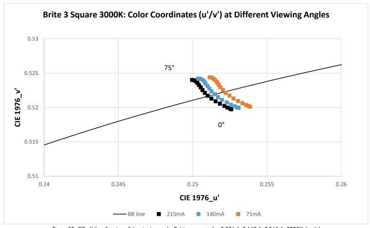
Figure 28: CIE u'lv' as function of the viewing angle. Driving currents I = 0.071 A, 0.140 A, 0.215 A, 3000K, level I
