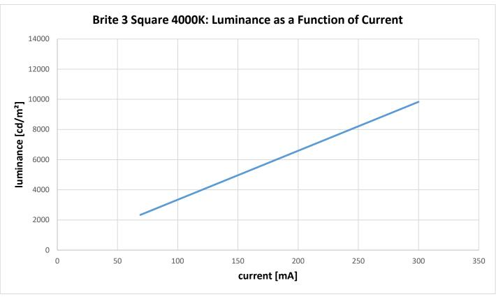
Figure 14: Luminance versus forward current at room temperature, Brite Square 4000K, level 1
