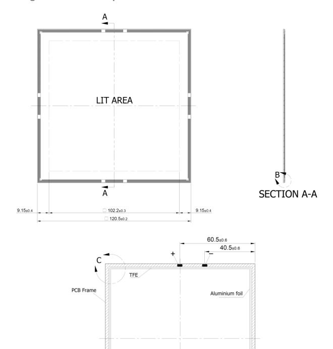
Figure 1: Brite 3 Square Level 1 – front and side view (top), rear view (bottom)
