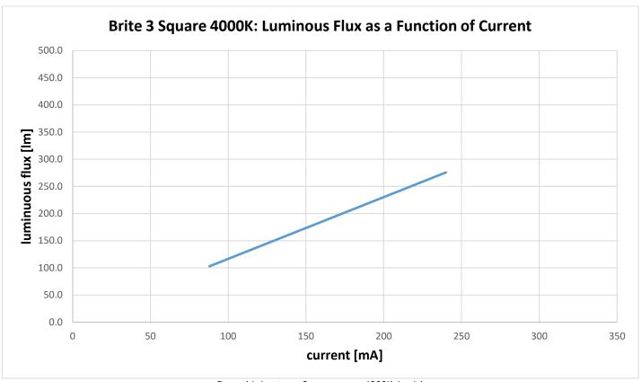
Figure 16: Luminous flux vs current, 4000K, level I
