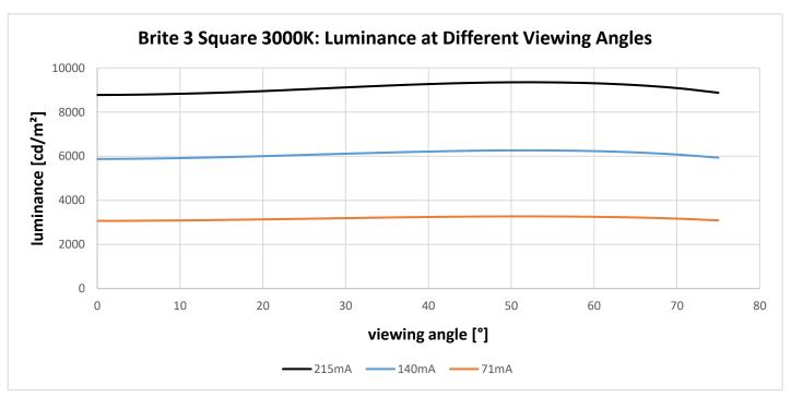
Figure 24: Luminance as function of the viewing angle. Driving currents I= 0.071 A, 0.140 A, 0.215 A, 3000K
