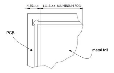
Figure 3: Detail C of Figure 1 - corner of PCB frame - Level 1
