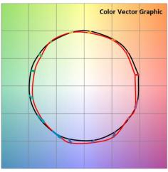
Figure 11: Color vector graphic based on TM-30 metrics for Brite 3 Square 3000K
