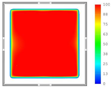
Figure 22: Typical luminance distribution for a Brite 3 Square Level 1. Operation conditions: vertical in air, RT (= 25 °C), I = I<sub>in rated</sub>
