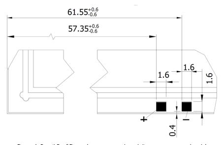
Figure 4: Detail D of Figure I – contact pads and distance to corner - Level I
