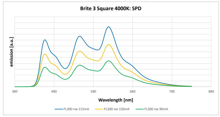
Figure 12: typical emission spectra of the Brite 3 Square 4000K at different driving currents (I = 0.090 A, 0.150 A, 0.215 A)
