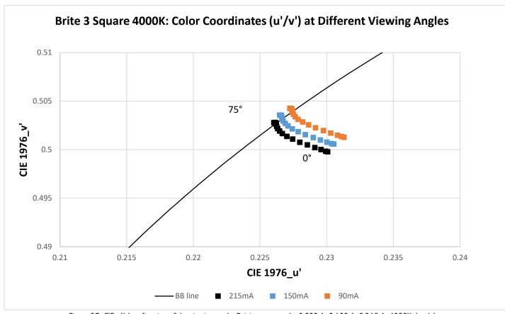
Figure 27: CIE u'lv' as function of the viewing angle. Driving currents I= 0.090 A, 0.150 A, 0.215 A, 4000K, level I
