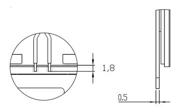
Figure 7: Details A and B of Figure 6 – solder orientation on PCB and thickness of metal back plate - Level 2
