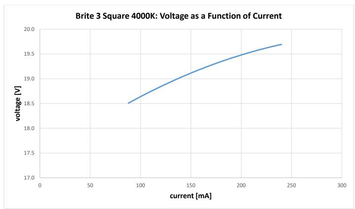
Figure 18: Voltage versus forward current at room temperature, 4000K, level  $\,\mathrm{I}\,$
