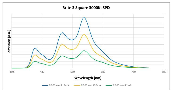
Figure 13: typical emission spectra of the Brite 3 Square 3000K at different driving currents (I = 0.071 A, 0.150 A, 0.215 A)
