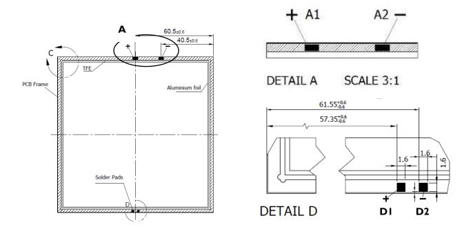
Figure 8: Contact pads of the Brite 3 Square Level I
