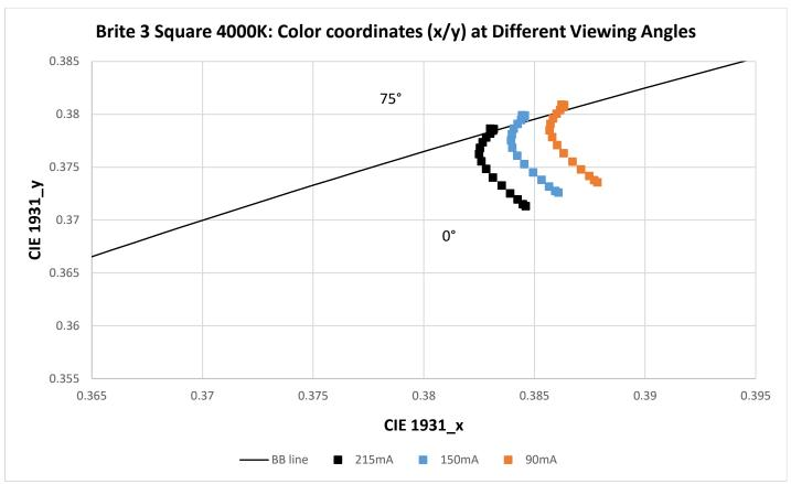
Figure 25: CIE x/y as function of the viewing angle. Driving currents I= 0.090 A, 0.150 A, 0.215 A, 4000K, level I
