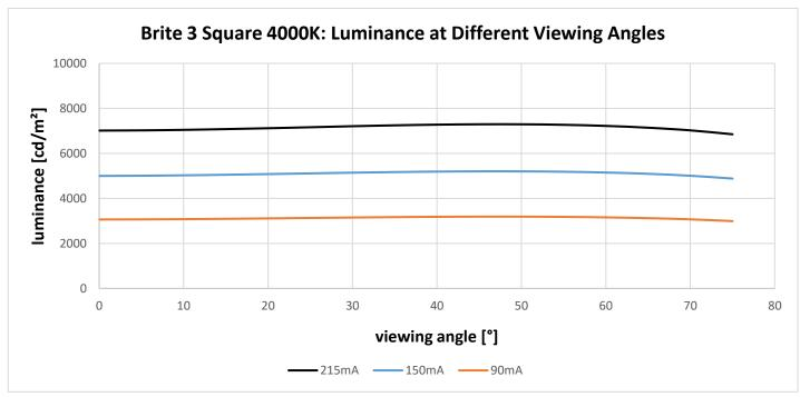
Figure 23: Luminance as function of the viewing angle. Driving currents I= 0.090 A, 0.150 A, 0.215 A, 4000K
