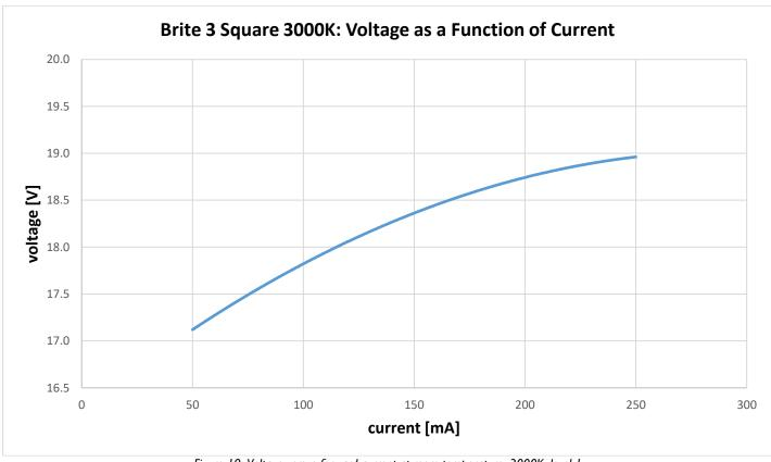
Figure 19: Voltage versus forward current at room temperature, 3000K, level 1
