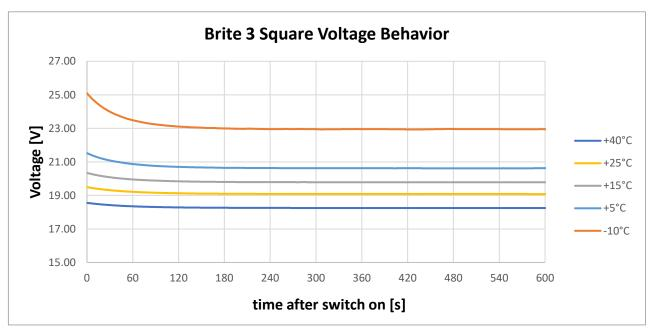
Figure 9: typical voltage evolution after start-up at different ambient temperatures, level 1, vertical orientation, air,  $I_{in rated} = 0.215 \text{ A}$
