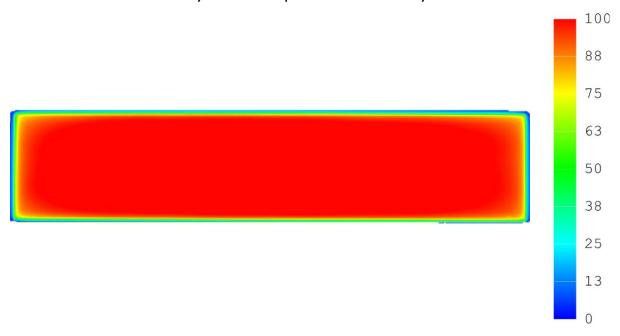
Figure 21: Typical luminance distribution for a Brite 3 Rectangle Level 1. Operation conditions: vertical in air, RT (= 25 °C), I = I<sub>in rated</sub>
