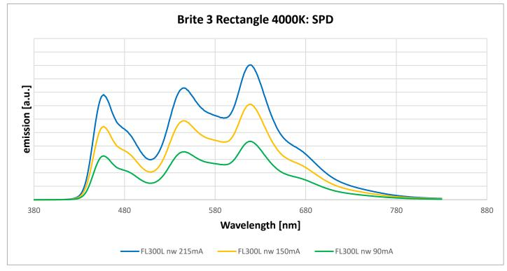
Figure 11: typical emission spectra of the Brite 3 Rectangle 4000K at different driving currents (I = 0.090 A, 0.150 A, 0.215 A)
