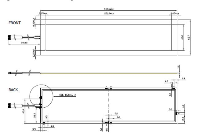
Figure 3: Brite 3 Rectangle Level 1.5 – front (top), side view (middle), rear view (bottom)
