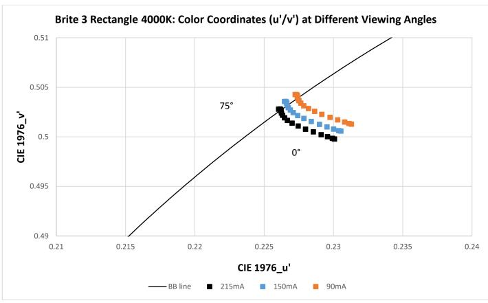
Figure 26: CIE u'/v' as function of the viewing angle. Driving currents I= 0.090 A, 0.150 A, 0.215 A, 4000K
