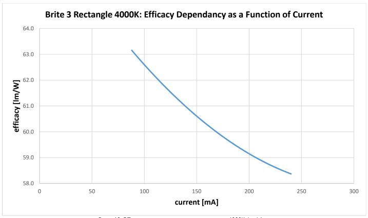
Figure 19: Efficacy versus current at room temperature, 4000K, level 1
