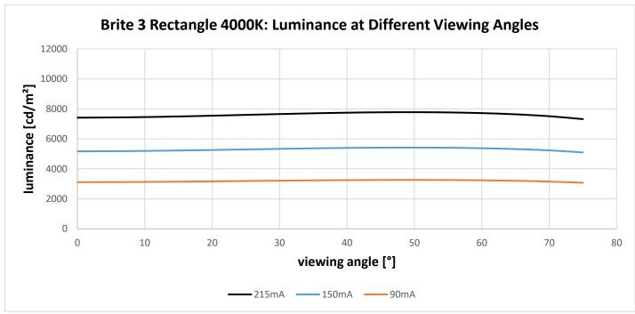
Figure 22: Luminance as function of the viewing angle. Driving currents I= 0.090 A, 0.150 A, 0.215 A, 4000K
