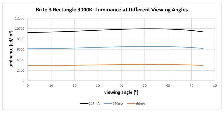
Figure 23: Luminance as function of the viewing angle. Driving currents I= 0.066 A, 0.140 A, 0.215 A, 3000K
