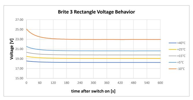
Figure 8: typical voltage evolution after start-up at different ambient temperatures, level 1, vertical orientation, air, Iin rated = 0.215 A
