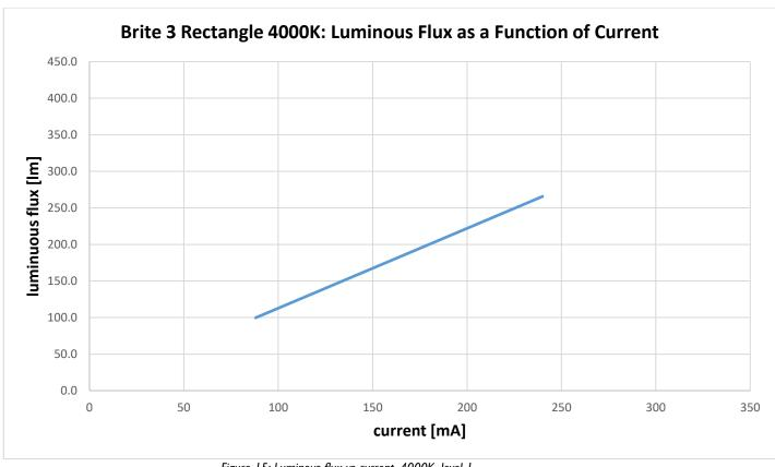
Figure 15: Luminous flux vs current, 4000K, level 1
