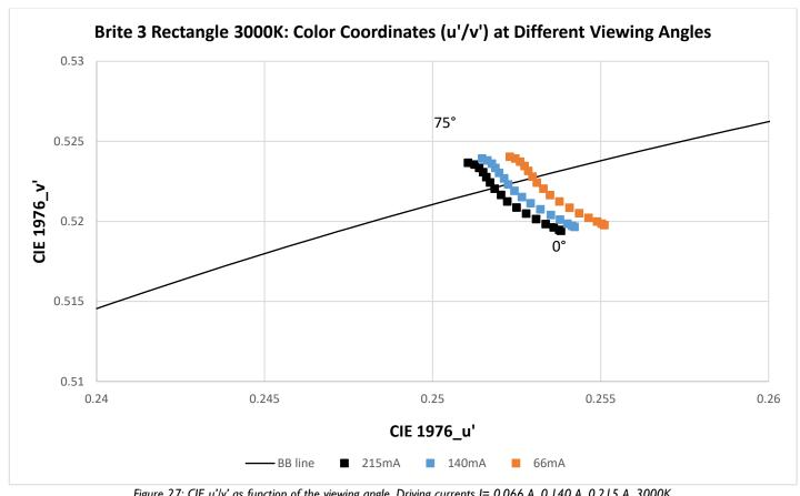
Figure 27: CIE u'/v' as function of the viewing angle. Driving currents I= 0.066 A, 0.140 A, 0.215 A, 3000K
