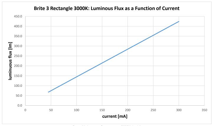
Figure 16: Luminous flux vs current, 3000K, level 1
