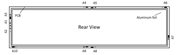
Figure 7: Contact pads of the Brite 3 Rectangle Level 1
