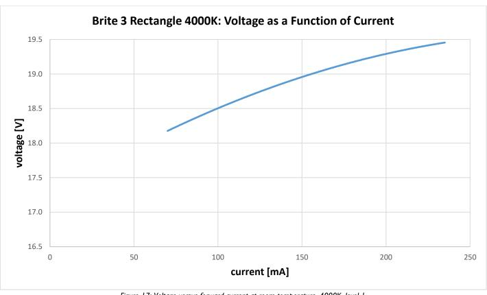
Figure 17: Voltage versus forward current at room temperature, 4000K, level 1
