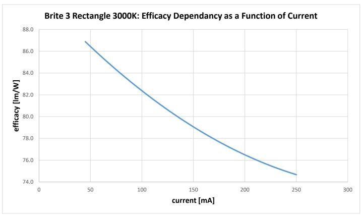
Figure 20: Efficacy versus current at room temperature, 3000K, level 1
