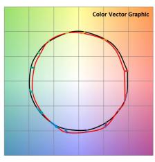
Figure 10: Color vector graphic based on TM-30 metrics for Brite 3 Rectangle 3000K
