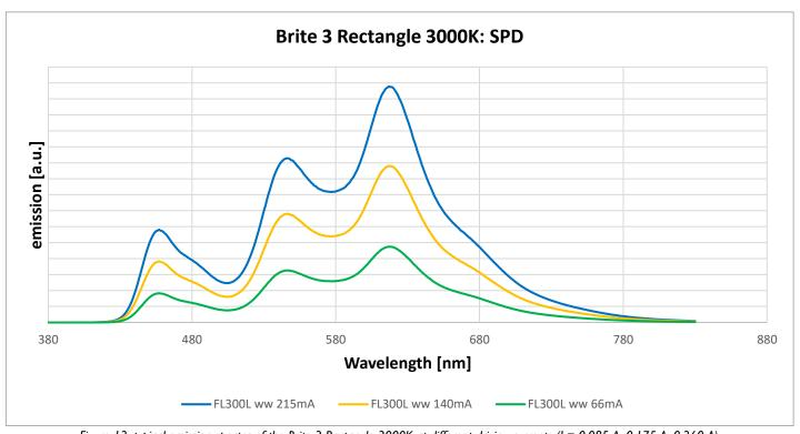
Figure 12: typical emission spectra of the Brite 3 Rectangle 3000K at different driving currents (I = 0.085 A, 0.175 A, 0.260 A)
