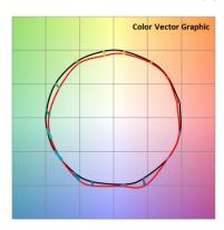
Figure 9: Color vector graphic based on TM-30 metrics for Brite 3 Rectangle 4000K
