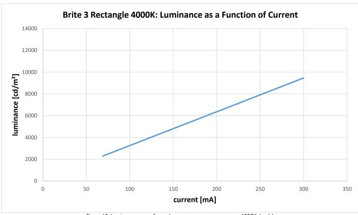
Figure 13: Luminance versus forward current at room temperature, 4000K, level 1
