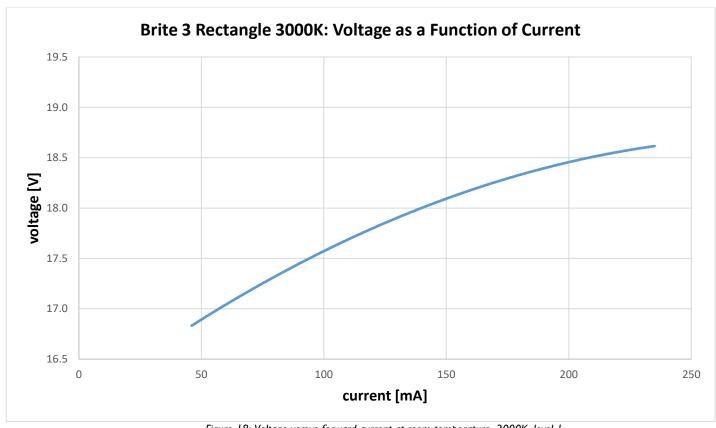
Figure 18: Voltage versus forward current at room temperature, 3000K, level 1
