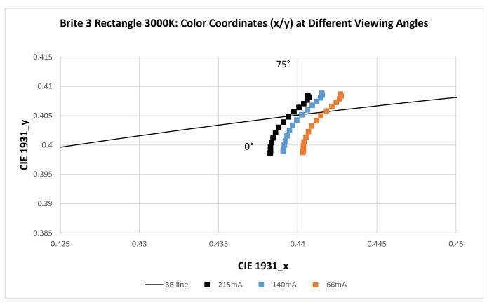
Figure 25: CIE x/y as function of the viewing angle. Driving currents I= 0.066 A, 0.140 A, 0.215 A, 3000K
