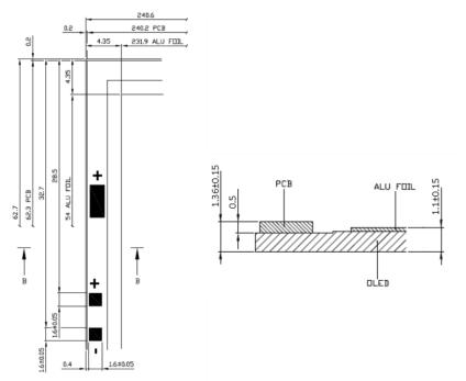
Figure 2: Detail A of Figure 1 (left) and cross section B-B (right); Brite 3 Rectangle Level 1
