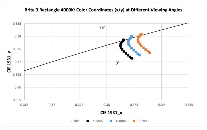
Figure 24: CIE x/y as function of the viewing angle. Driving currents I= 0.090 A, 0.150 A, 0.215 A, 4000K
