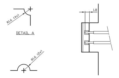
Figure 6: Details A and B (screw openings) and view C-C (solder orientation on PCB) of Figure 5 – Level 2
