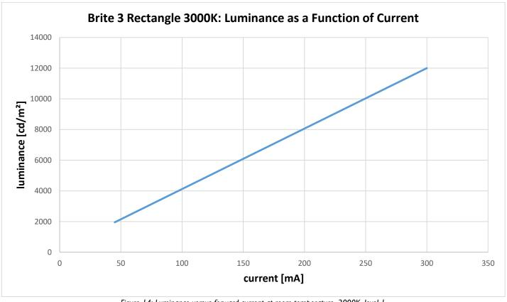
Figure 14: Luminance versus forward current at room temperature, 3000K, level  $\,I\,$
