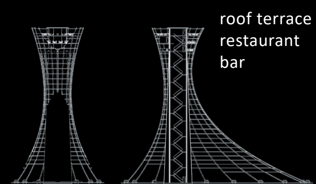
two glass elevators and a double emergency stairwell cross section longitudinal section Sections
