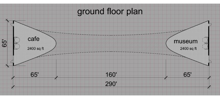
In the wings of the arch, 2 rooms are formed with an area of 2,400 square feet each. One can house cafe, and another the Electric Tower Museum with Tower model on a scale of 1:4. There are 2 rows of rails under the ceiling of the arch for suspended cabs on which the visitor can drive from one room to another, observing the unusual interior of the arch and the surroundings from a height of 140 feet.
