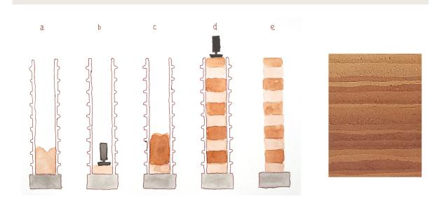
A scheme for erecting a wall using rammed earth technology. Different layers of the rammed earth monolithic wall are marked with different colors. Steps when erecting a wall: (a) Formwork is built and filled with a layer of moist soil-cement mixture. (b) The layer of moist mixture is compressed. (c) The next layer of moist soil-cement mixture is added. (d) Successive layers of moist earth are added and compressed. (e) The formwork is removed leaving the monolithic wall.
