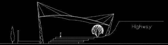
The roofed amphitheater is placed at the northeast part of the site which most of its seats have a good view to the main tower in the background. the roof is to protect from sunlight and rain. However it was inspired to reduce the noises from the highway.
