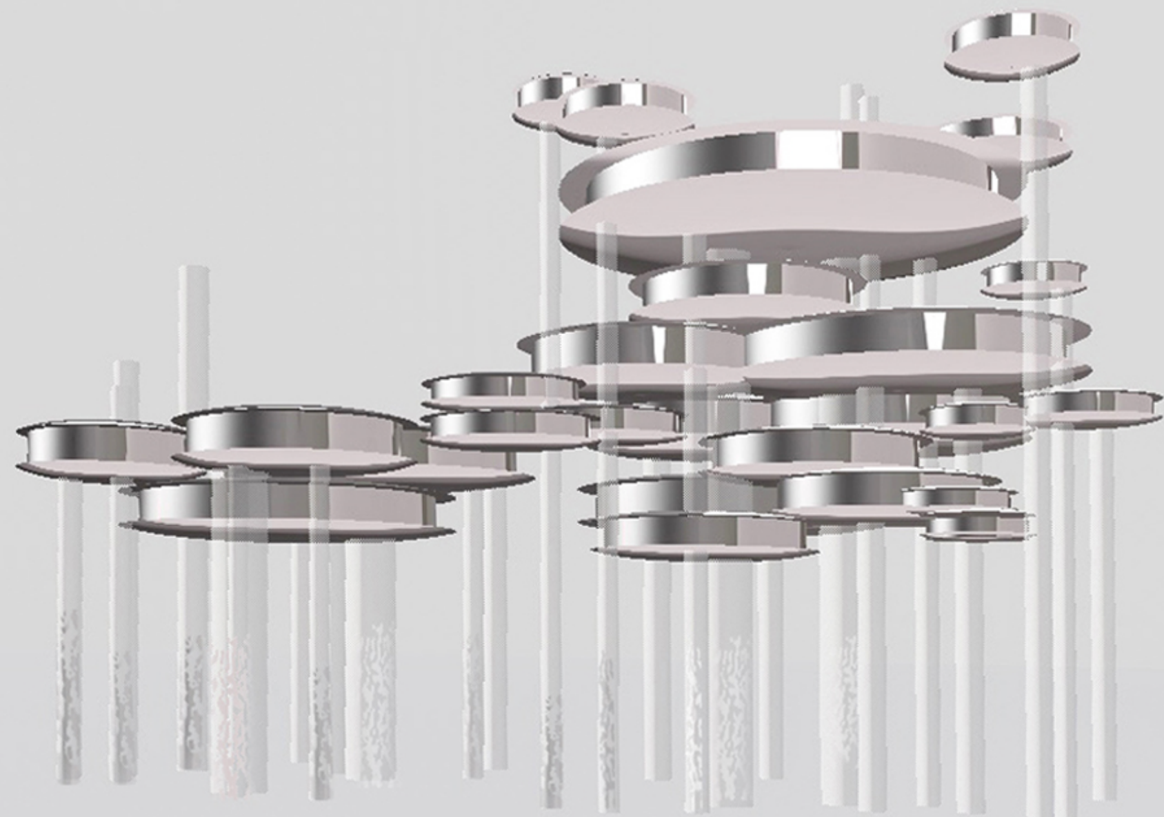
Height: 200 feet Width: ca 230 feet Panoramic disks vary in size and curvature Largest about 100 feet wide
