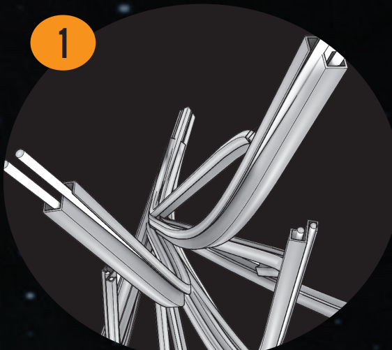
1 Controllable LED strip light channels encased within CFRP sections.
