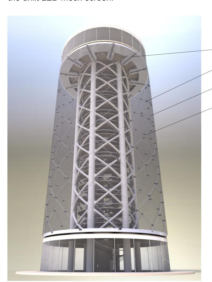
**Upper Actuators** Cable Structure LED Mesh Screen **Swarm Robots**
