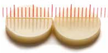
Initial appearance and after 10,000 brushing cycles
