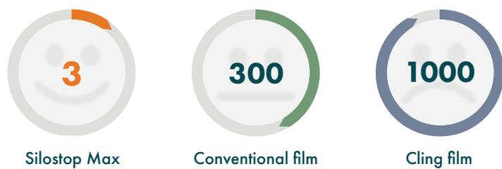
Test results shown above are approximate and are based on DIN 53380-3 showing oxygen transmitted in cm³/m²/24h at 21% O₂ and 50% relative humidity
