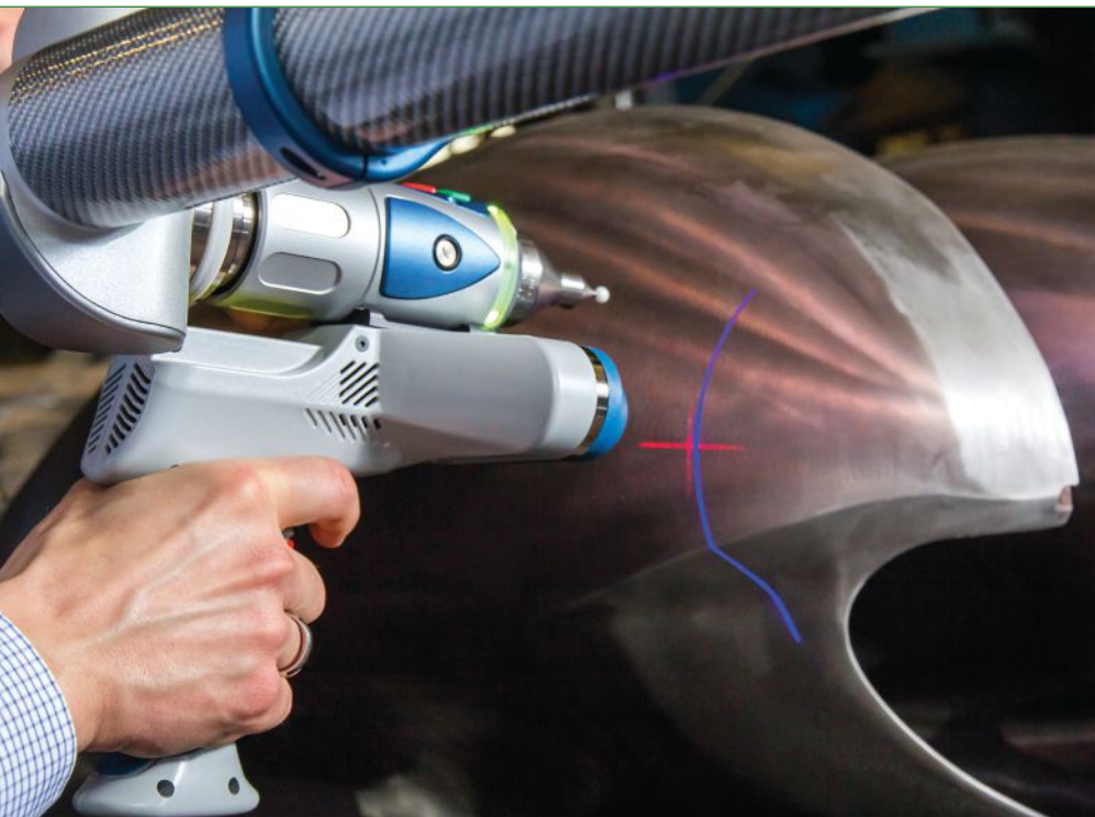
Precise Tooling Solutions uses a FaroArm with surface plates to inspect parts.
