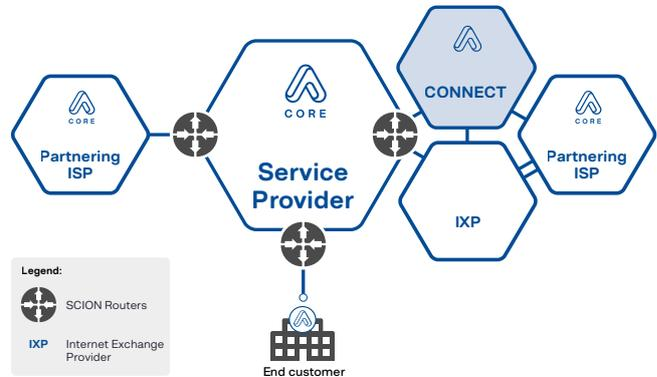
Once Anapaya CORE is installed within a service provider, any clients can access and use the SCION-Internet via Anapaya EDGE, the end-user gateway to access the SCION-Internet.
