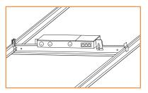
Secure the junction box to the linear light and tighten the two terminal nuts.
