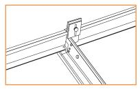
Turn off the main power. Install the linear light to the ceiling grid and tighten two terminal nuts.
