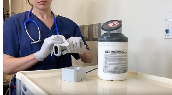
Hospitals are migrating to patient-care tools, such as barcode readers, made from disinfectant-ready plastics that withstand near-constant disinfection.
