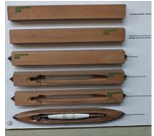
The stages in making a hand-threaded shuttle
