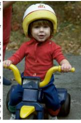
This type of trike is not as easy to handle for a young child just learning to steer and pedal, due to its awkward steering geometry. They have an extremely shallow head angle, which makes the wheel tend to flop to one side or the other too easily.
