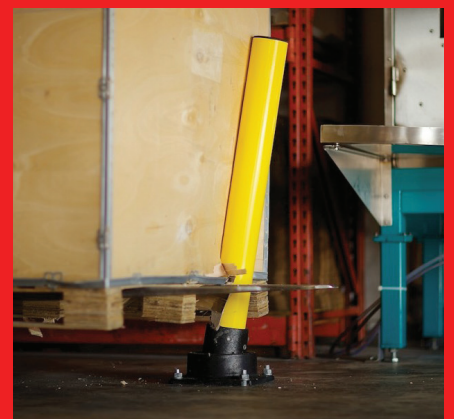
Slow Stop Bollards under forklift impact
