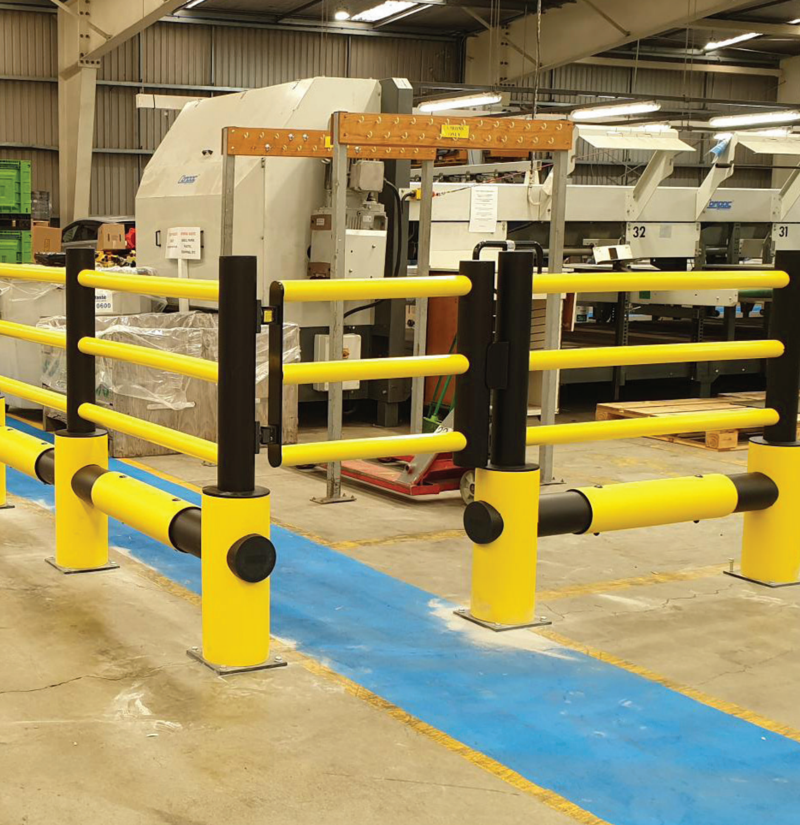
d-flexx Flexible Barrier System for guiding pedestrian traffic and protecting from moving vehicles - Seeka Oakside, Bay of Plenty
