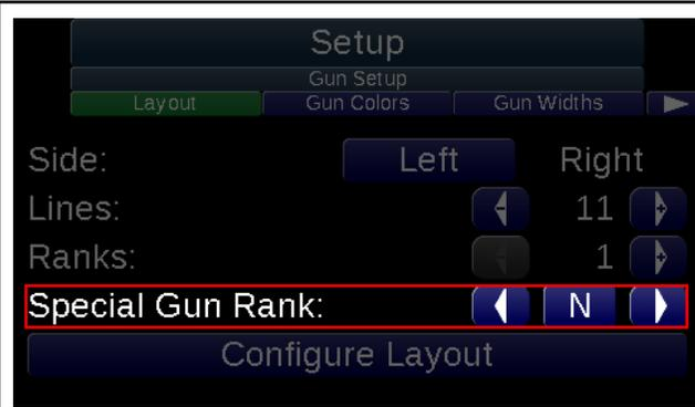
Press the **Configure Layout** button to enter the screen for specifying the paint gun positions.
