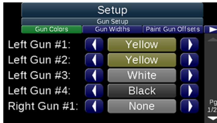
**Gun Colors** sets the color for each gun. Note that proper color setting is important for accuracy in mil thickness calculations, pump control features, data logging, and report printouts.
