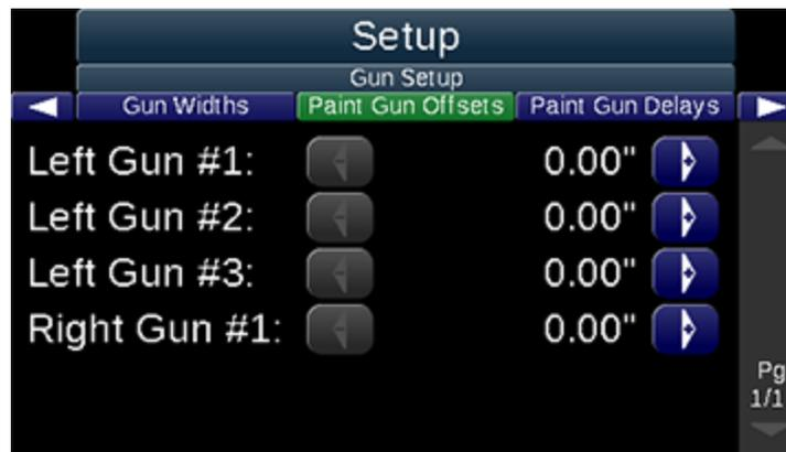
Set **Gun Offsets** for all items in the gun line, including *Paint, Beads, Tandem Beads, or Blow Air*. Only available guns will appear in the **Gun Setup** menu.
