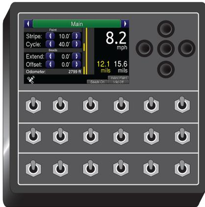
The **Master Control Box** provides the primary interface for the operators. It includes a full-color character LCD display menu along with toggle switches that together define the striping patterns and operation.
