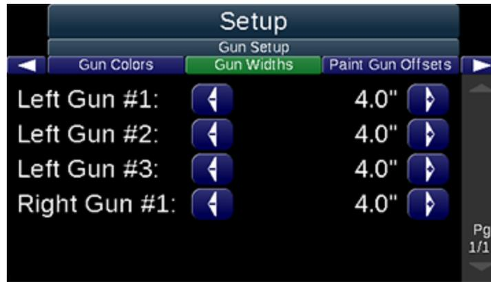
**Gun Widths** sets the gun widths to match the actual application width of the material on the road.
