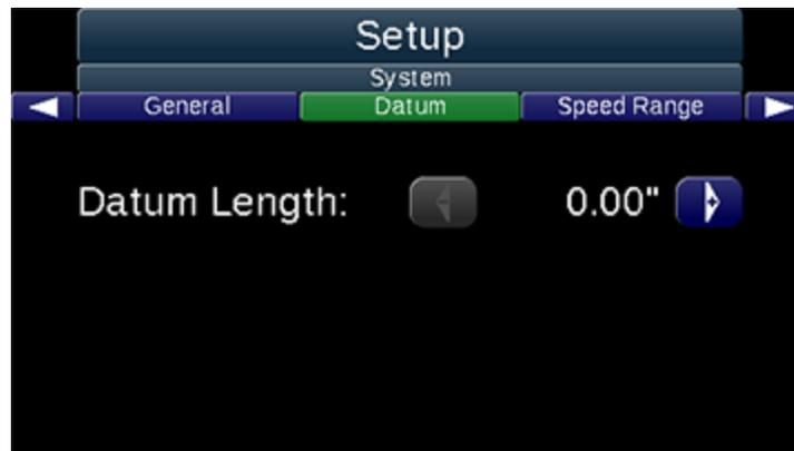
**Datum Length:** The **delay** distance in front of the first gun, the point where the pattern will actually begin. Refer to section 5.2, **Datum Point** for more information.
