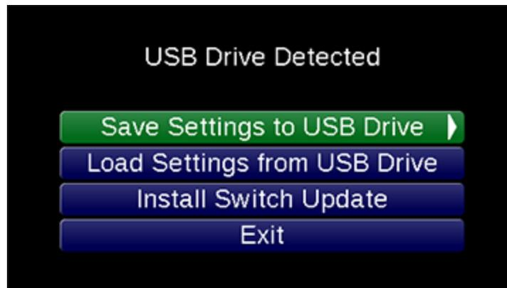
The USB menu appears when a USB drive is inserted. It is primarily used to export Counter Channel data, although future USB functionality may be here as well. *For more information, see the 5.1, **Counter Channel Logging**.*
