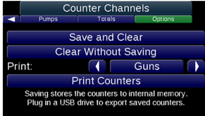
The logging feature records the counter channels when they are cleared. The typical use case is for the operator to:
