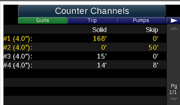
The **Trip Counter** feature acts like the trip odometer on vehicles. Any trip counter can be cleared individually, but the regular counters will remain intact, preserving job footages and application rates.
