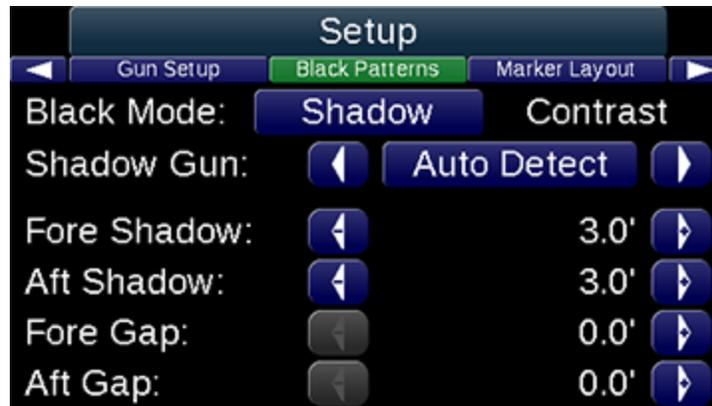
**Black patterns** cause the special Black Gun to have specific behavior. On some skip timers, this is configurable. On others, the special Black Gun behavior is fixed to Gun #4. Physical mounting of the black material gun is important when using this special mode. Refer to the **Pattern Preview** area on the **Main screen** to see the expected pattern.
