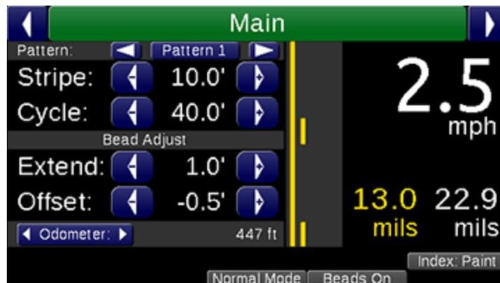
The Main Screen is the recommended screen to use during striping operations. It is organized into several sections.
