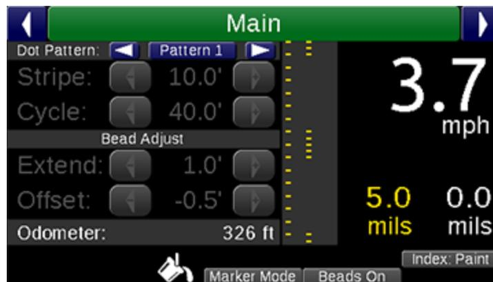
**Marker layout mode** can be enabled on the **Quick Setup** menu (see 4.3.1, **Mode**). When enabled, the main screen Stripe and Cycle parameters are disabled.
