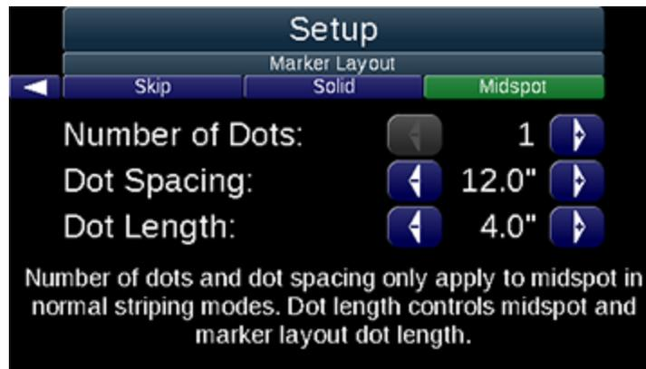
Dot Length controls the length of the dot, in inches. Set it to a length sufficient for the paint gun to emit material at the desired vehicle speed.
