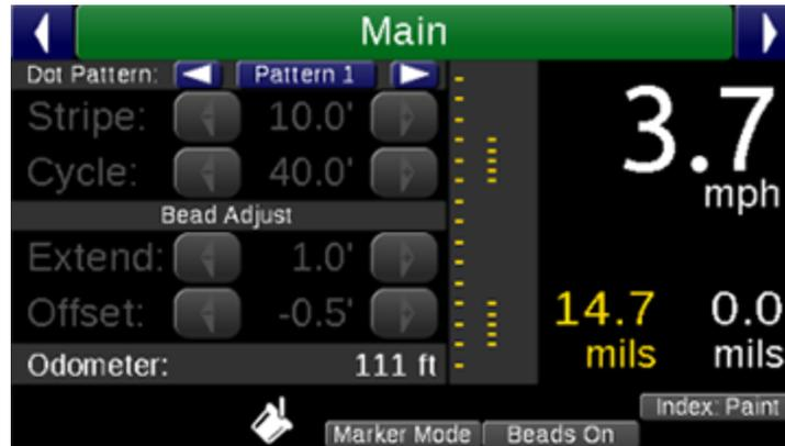
Create the desired pattern by setting the distance between markers in the Skip and Solid pattern sub-menus.
