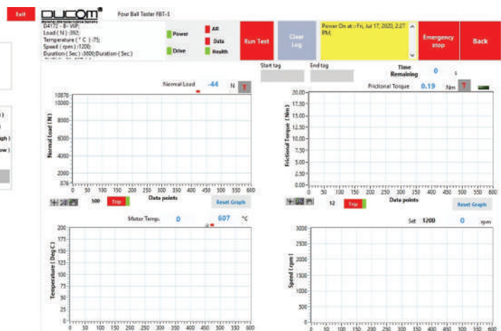
Figure 6. Data acquisition screen with live data in LabVIEW based WinDucom software in FBT-3.
