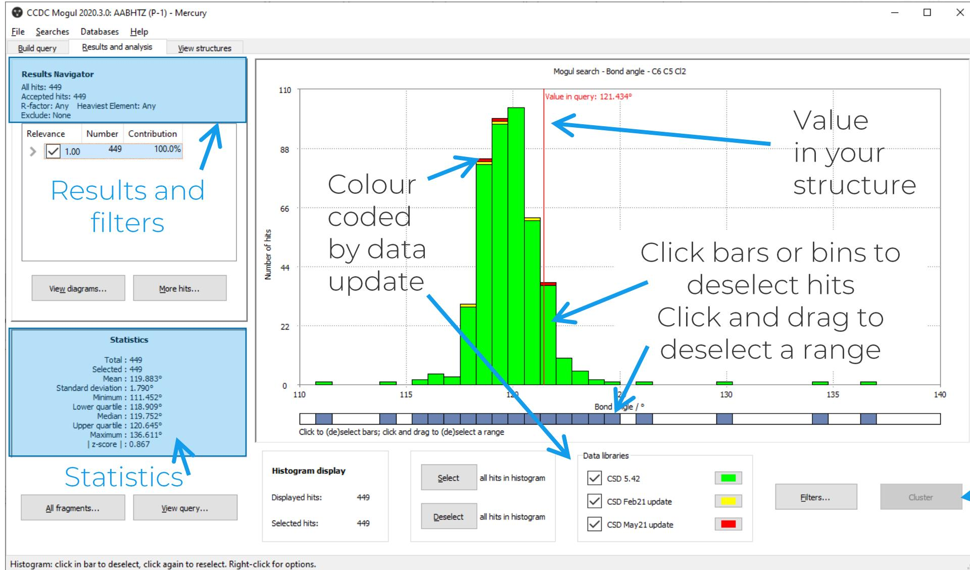
Histogram built with data from structures in the CSD
