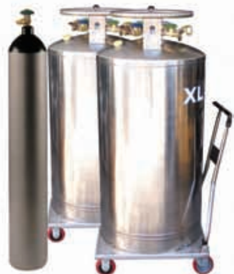
High pressure CO 2 cylinder, L-CO 2 and L-N 2 dewars with 'trolleys' makes moving the dewars very easy
