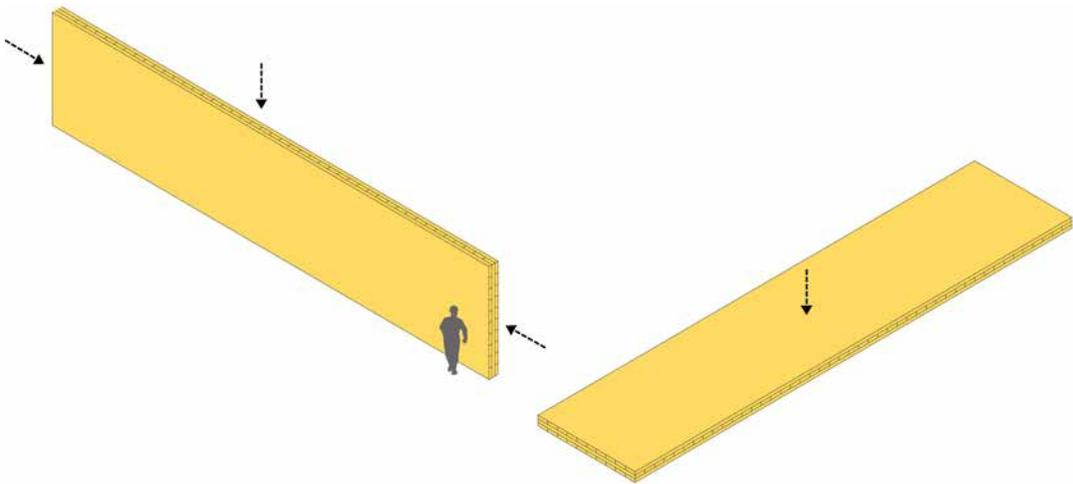
CLT can resist load both as a beam (ie. in-plane), or a slab (out-of-plane)
