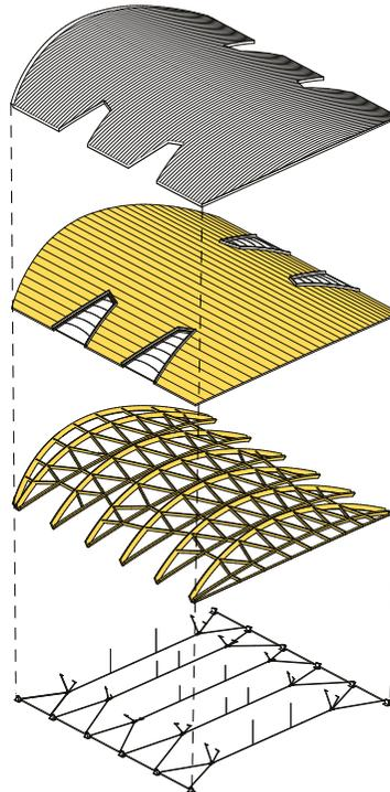
Exploded Diagram of Roof Structure
