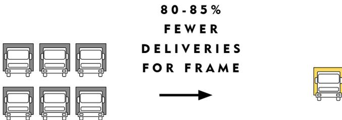
The light weight and prefabricated nature of CLT construction typically offers an enormous reduction in the number of deliveries to site, compared with concrete frame, especially when schemes are designed with an understanding of delivery parameters. In comparison to in-situ concrete frames, around 80-85% fewer deliveries are required for a CLT structure, greatly reducing the impact of site logistics on the surrounding community.<sup>3</sup>
