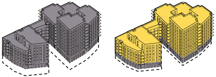
The diagram indicates an approximate reduction in the raft foundations required for a CLT version of the Dalston Works scheme.
