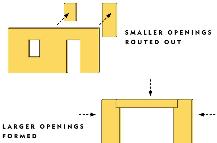
Where particularly large openings are needed it can be more cost effective to form openings from multiple pieces of CLT. The benefits should be considered against the additional lifts on site and additional joints that can increase the construction period and have the potential to reduce accuracy and structural performance.
