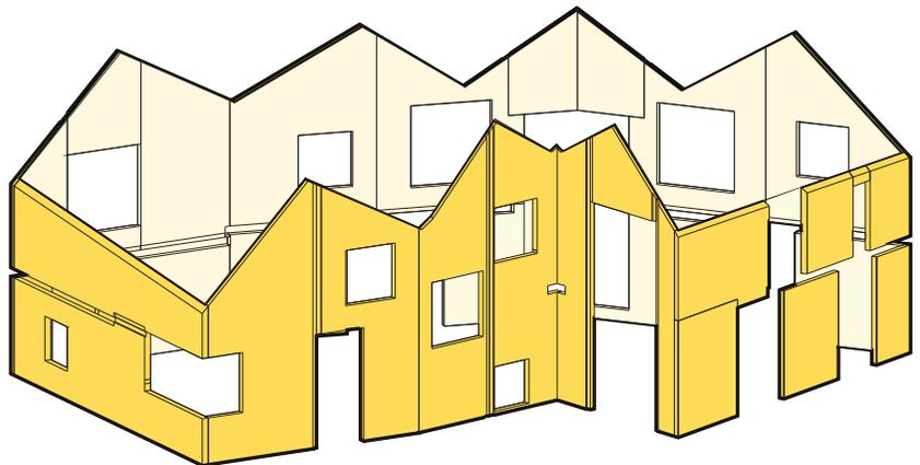
Isometric CLT Panel Diagram
