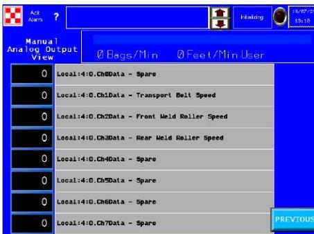
(fig.34) Manual Analog Output View 13-23
