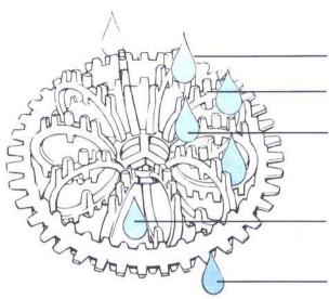
Liquid is collected by inertial impaction.
