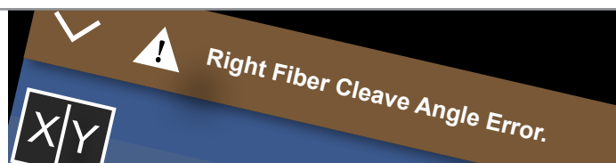
Figure 1. According to SumiCloud™ splice data, approximately 15% of fiber preparations are rejected by the splicer because of poor cleaves.
