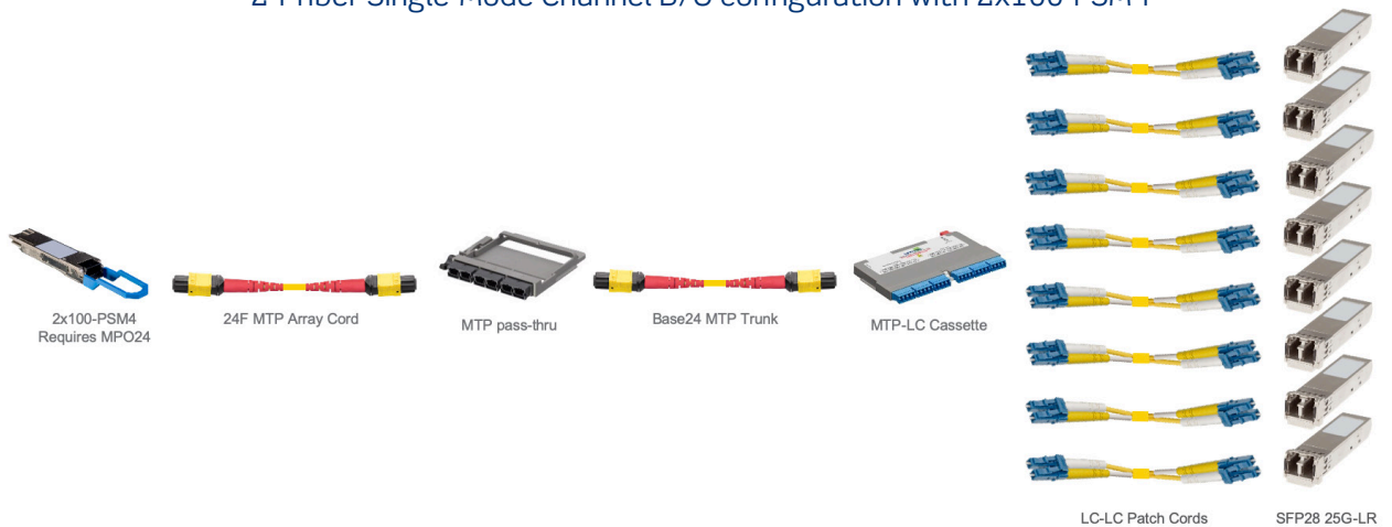
Figure 9: 200G to 8x25G Breakout Use Case 24-fiber Single-Mode Channel B/O configuration with 2x100-PSM4
