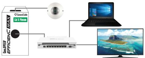
\* 0.6A is the amapcity rating of the cable, which equates to 120 watts using 50 volts over four pairs.
