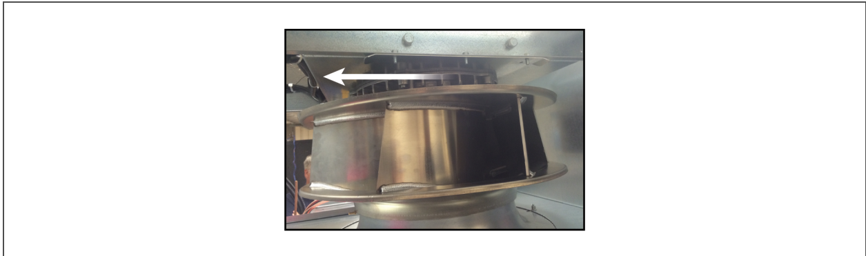
Figure 8.7 Slide the fan assembly out the front of the unit
