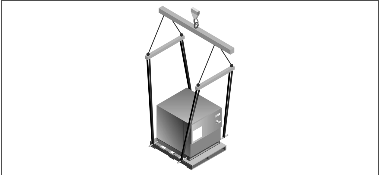
Figure 5.3 Typical sling arrangement for lifting unit
