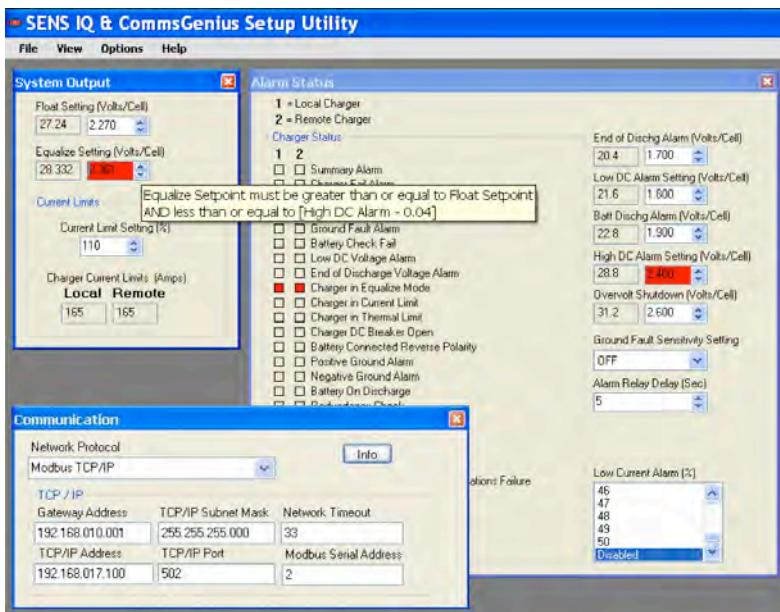
SENS *Setup Utility* is a PC-based application that communicates with the charger over USB. It is included with the Modbus communications option and the forced load share & remote temperature compensation package.
