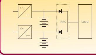
This schematic illustrates how the Best Battery Selector operates. Listed below are the applications where the Best Battery Selector is best suited for:
