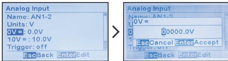
To adjust the high scale value assigned to the analog input:
