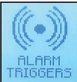
This icon is used to exclude alarms from the Common Alarm activation list. By default, all alarms, when active, will annunciate the Common Alarm.
