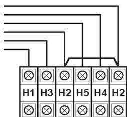
Before you connect ac power to ATevo, inspect the present ac input voltage setting, and confirm the correct jumper positions for the desired ac input supply voltage. The multi-tap ac input voltage setting can be verified without removing the safety shield.
