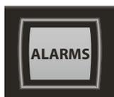
The ALARMS button displays the ATevo Active Alarm List, four (4) alarms per page. If more than four (4) alarms are active, use UP and DOWN arrows to scroll through the list.
