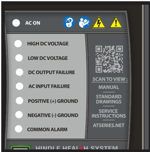
The **GREEN** AC ON LED indicator, and the six (6) **RED** Legacy Alarm LED indicators are summarized in the two-page table in Section 7.3, which identifies:
