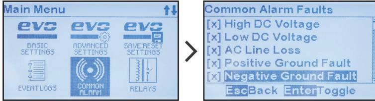
If an '[X]' appears to the left of the alarm, it will activate the COMMON ALARM. If '[' appears, it will not activate the COMMON ALARM.
