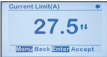
After setting the Current Limit level to the desired value and pressing EDIT/ENTER to save the set point, configuration of Basic ATevo Set Points and Alarms is complete. The display returns to the HOME screen.
