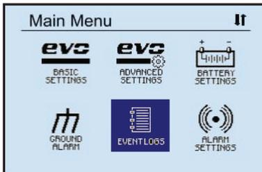
The top-left of the screen indicates the **Main Menu** displayed. The top-right displays an up and/or down arrow icon that indicates that more menu selection icons are available if you continue to navigate in the direction of the arrow(s). In the screen shot above, both up and down arrow icons appear in the top-right corner. This indicates that menu icons can be accessed by navigating either up or down from the presently selected icon.
