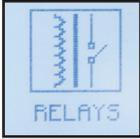
This icon shows relay configuration and control options. Use it to configure relays and reset or clear any latched alarm relays. To change a relay configuration, execute the 'Relay configuration' command then select the relay to configure.
