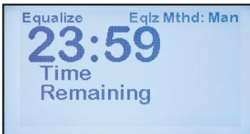
ATEvo will remain in EQUALIZE mode until either the EQUALIZE TIMER expires or the charge mode is manually switched back to FLOAT.
