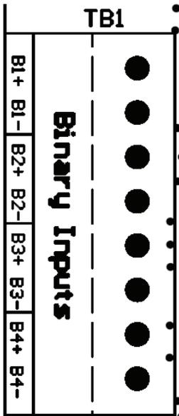
The terminal connections are labeled along the edge of the Auxiliary I/O Board next to terminal block (A4-TB1). Each binary input is optically isolated and has a polarized pair of terminals. Observe the pos(+) and neg(-) designators when wiring the terminal block.
