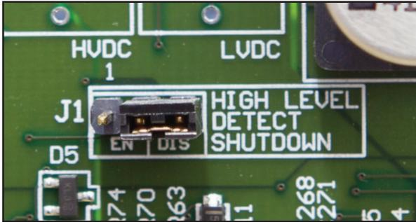
The High Voltage Shutdown jumper (J1) is located center-right, on the Main Control Board (A1).
