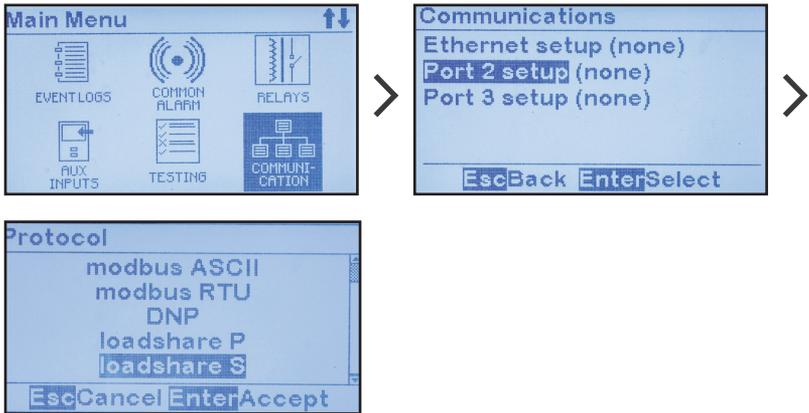
Press the EDIT/ENTER button to accept the new selection. The charger ID may now be changed. Press the ESC button to return to the previous screen. If a port setting was changed, the ATevo will prompt to RESET. Select YES to RESET the ATevo. The new port settings will not become active until after the ATevo is RESET.
