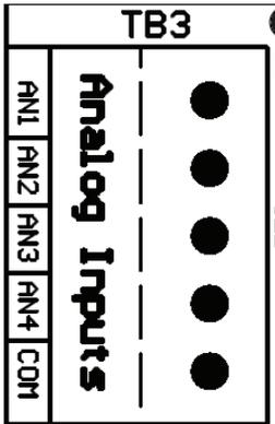
Terminal connections are labeled along the edge of the Auxiliary I/O Board next to terminal block (A4-TB3). The analog inputs are **NOT** isolated, and must be referenced to the negative (-) dc bus.
