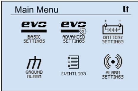
The top of the screen indicates the Main Menu is being displayed and to the far right of 'Main Menu' an up and/or down arrow icon is displayed. The arrow icon(s) indicate that more menu selection icons are available if you continue to navigate in the direction of the arrow.
