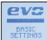
This icon opens Basic Set Points and Alarms screens beginning with the first parameter. These are the legacy AT10.1 settings. Refer to Section 4.2 for configuration instructions.
