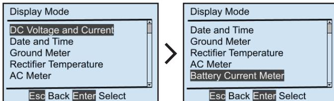
**NOTICE** The DISPLAY MODE button is in the same relative location as the METER MODE button on legacy AT10.1 Series battery chargers. Its functionality is equivalent, in that it determines which measurements are displayed on the HOME screen.
