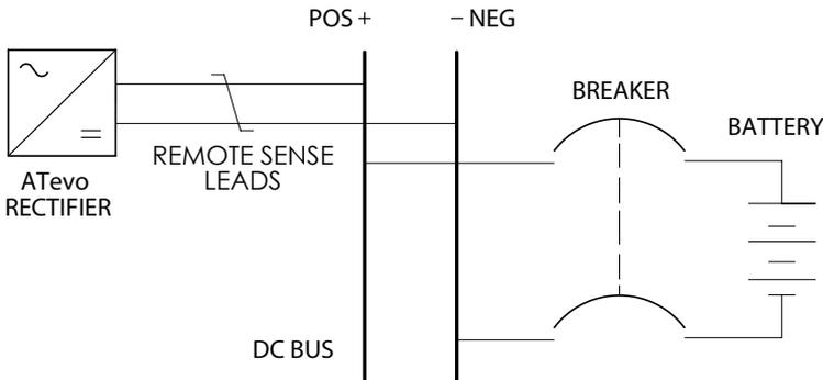
To wire ATevo for remote sensing, install twisted-pair cabling from the remote sense terminals to the battery terminals or dc bus. ATevo control circuitry measures dc voltage at the battery terminals and controls charger output to maintain battery voltage at the desired float or equalize voltage.
