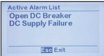
The Active Alarm List can display up to four (4) active alarms at once, but it is scrollable to view any additional alarms present.
