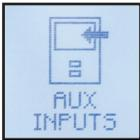
This icon configures binary inputs and analog inputs for up to four (4) Auxiliary I/O Boards. Each board may have up to four (4) generic binary inputs and four (4) generic analog inputs. Refer to Section 12.5 for binary inputs, and Section 12.6 for analog inputs.
