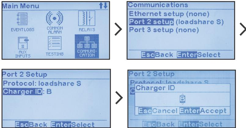
Press the EDIT/ENTER button to accept the new selection. Press the ESC button to return to the previous screen. If a port setting was changes, the ATevo will prompt to RESET. Select YES to RESET the ATevo. The new port settings will not become active until after the ATevo is RESET.
