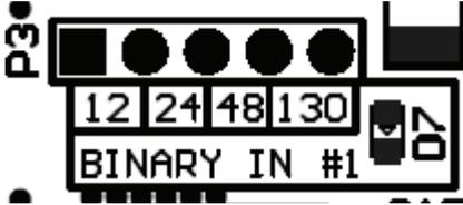
To configure binary input voltage, move the SHORTING BLOCK to connect the two (2) header pins directly above the voltage rating (12, 24, 48, or 130). Factory default jumper setting is 130. Repeat this process for the remaining three (3) binary inputs, using the associated configuration jumpers for Binary Input #2, #3, and #4.
