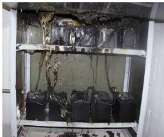
An example of a battery after thermal runaway
