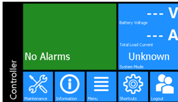
Figure 8 — CXC HP Controller Touchscreen Display
