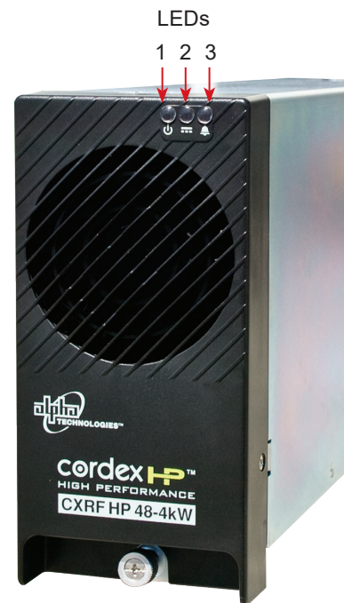
Figure 11 — Cordex HP 4.0k Rectifier Front Panel LEDs
