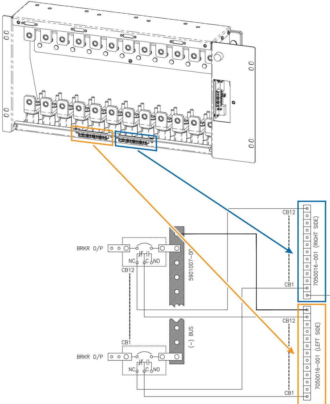
Figure 49 — High Capacity Breaker Panel Alarm Wiring
