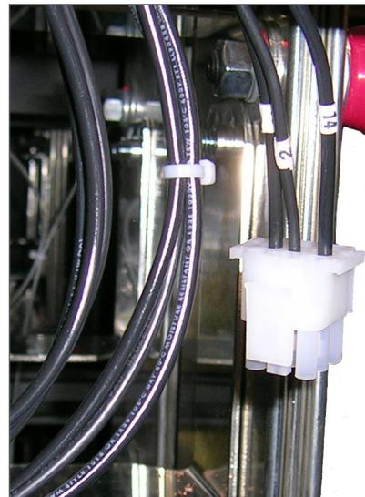
Figure 33 — Inter-bay Wiring Harness
