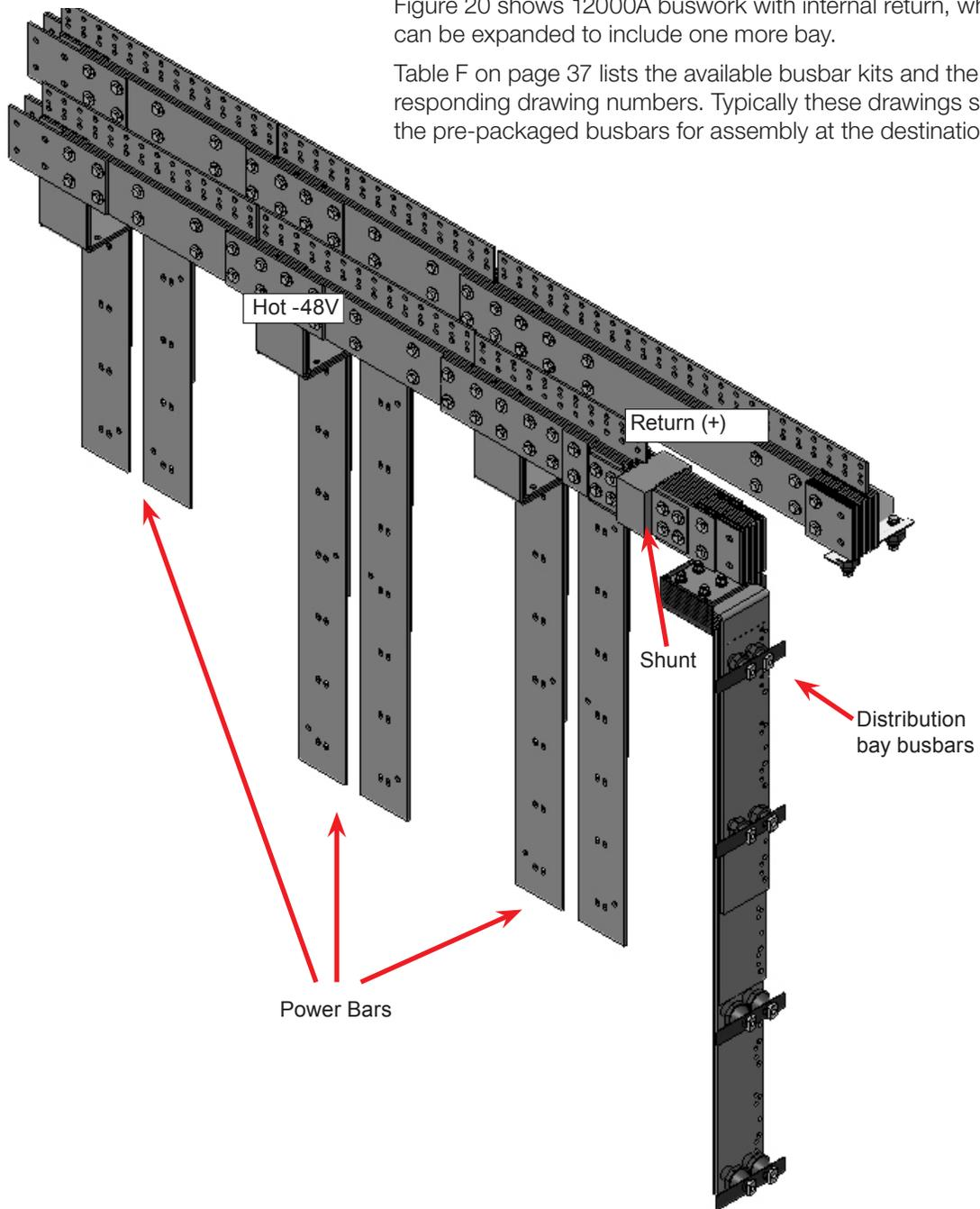
Figure 20 shows 12000A buswork with internal return, which can be expanded to include one more bay.
