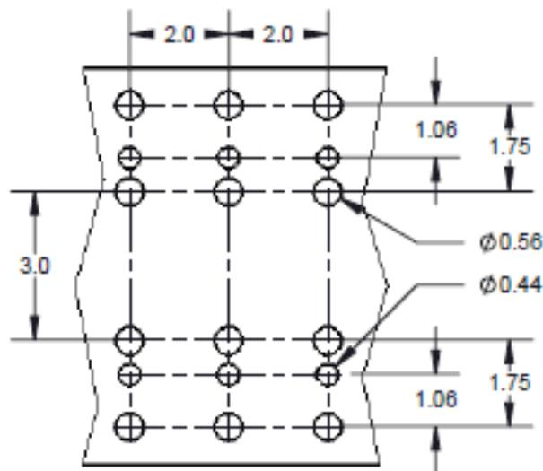
Figure 51 — Customer Connections Spacing
