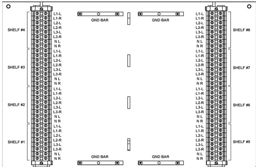
Figure 47 — Terminal Blocks for 16-feed 208/480Vac input
