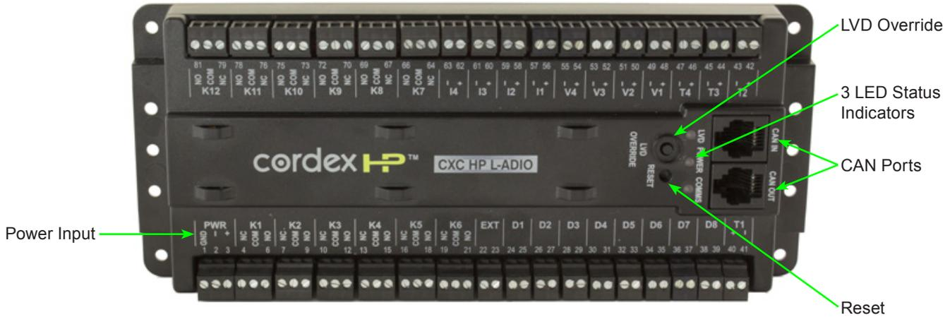
Figure 24 — L-ADIO I/O Peripheral
