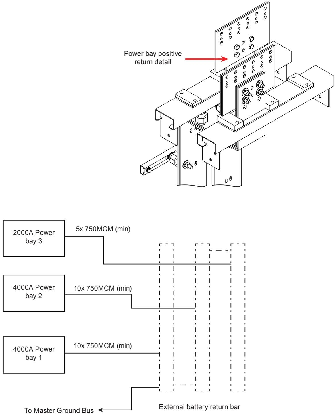
Figure 50 — External Battery Return Bar Wiring
