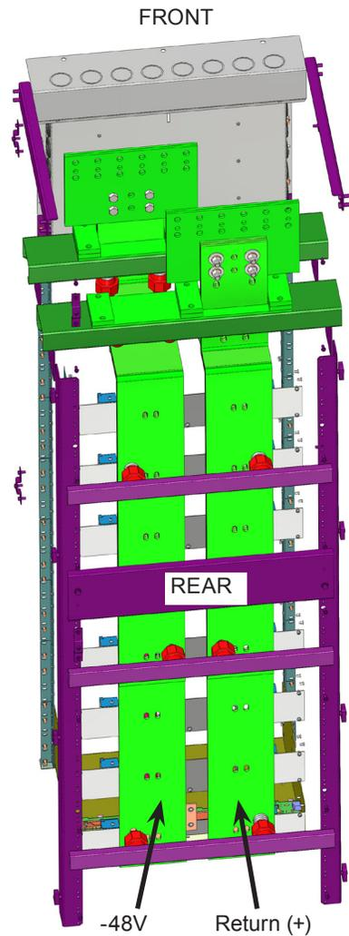
Figure 3 — Stand-alone Power Bay showing DC Charge Buses
