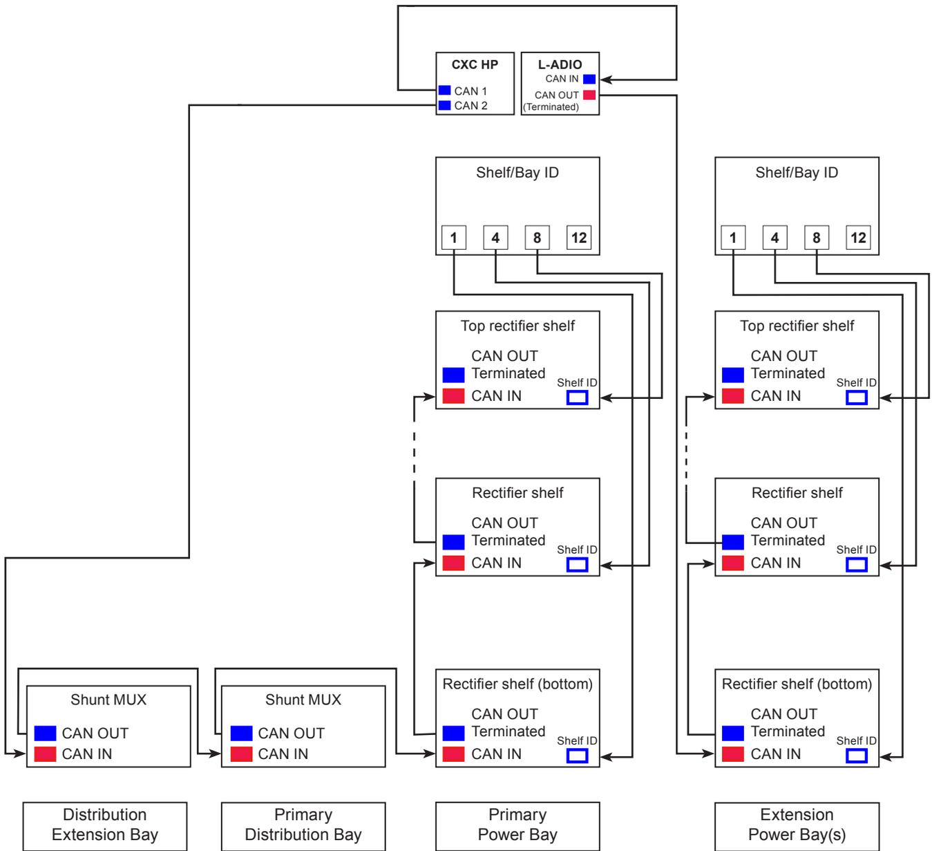
Figure 36 — Controller and Shelf/Bay ID, CAN Bus and Shelf ID cabling
