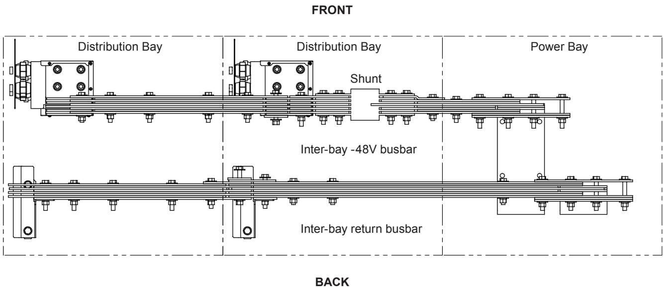
Figure 4 — Top View of Horizontal Inter-bay Busbars
