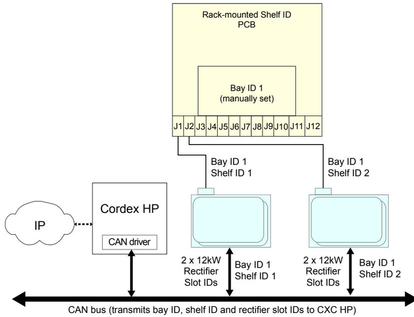
Figure 52 — Example of a Single Bay with Two Rectifier Shelves.
