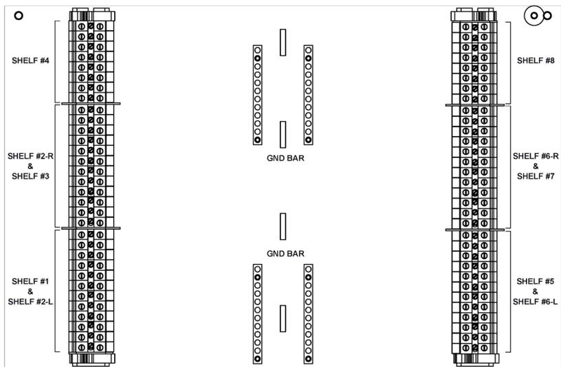
Figure 48 — Terminal Blocks for 6-feed 480Vac input
