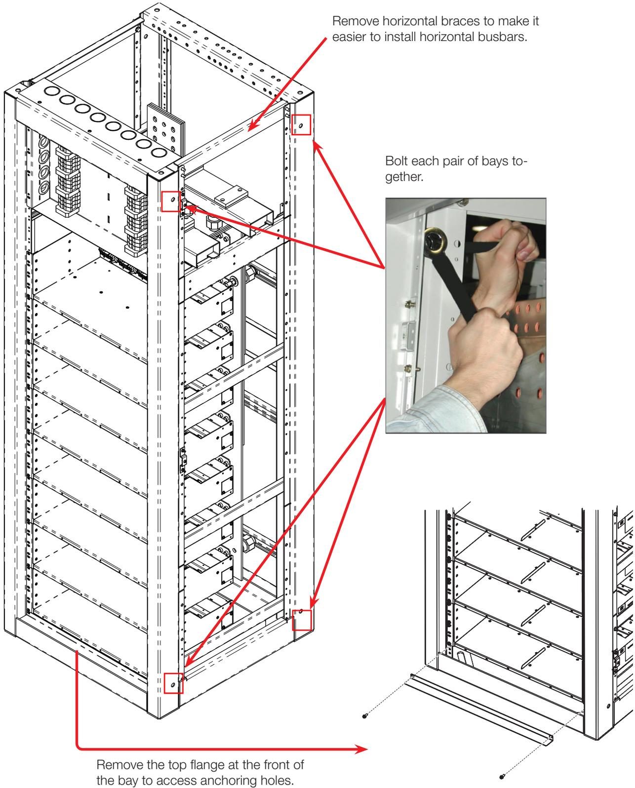
Figure 30 — Bolting Adjacent Bays Together
