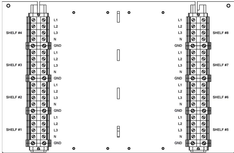
Figure 46 — Terminal Blocks for 8-feed 3 wire 208/480Vac input
