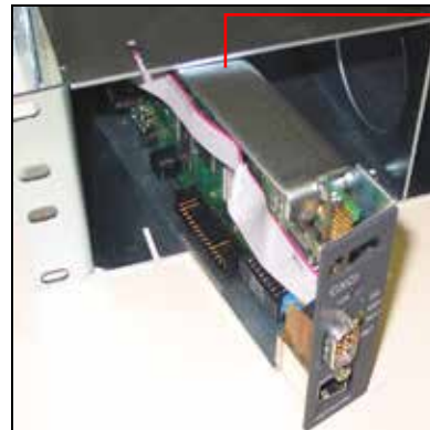
Figure 13–Showing CXCI module removal (replacement)
