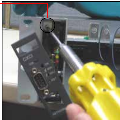
Figure 13–Showing CXCI module removal (replacement)
