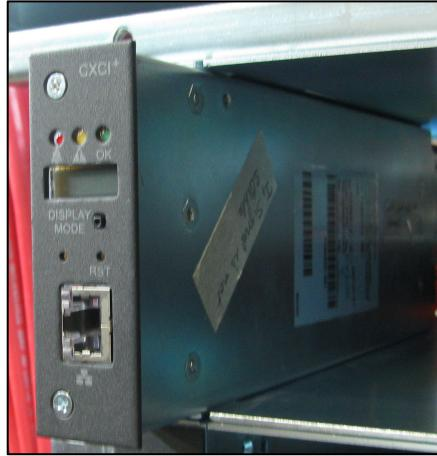
**Figure 17–Showing CXCI+ controller module replacement**
