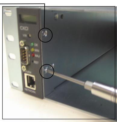
Gently remove the LCD to access the front mounting screw
