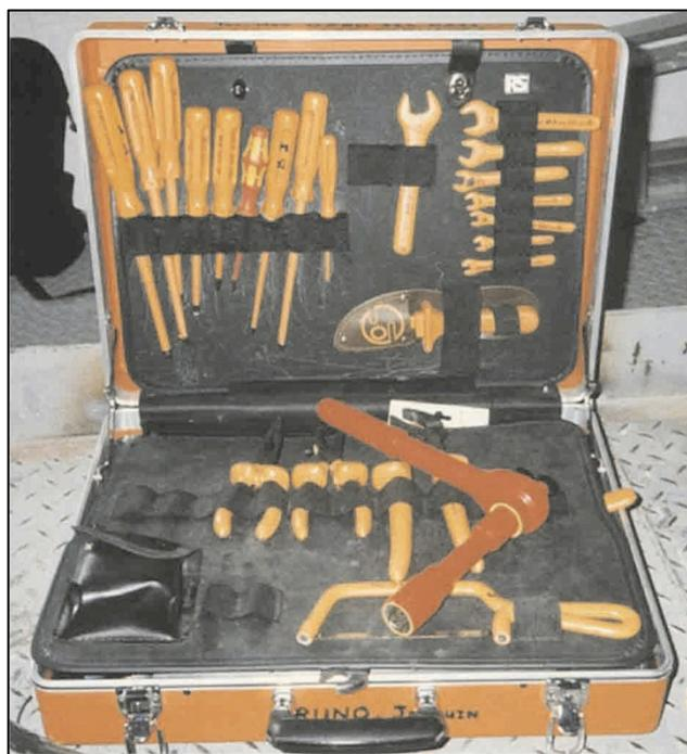
Figure 9—Example of an insulated tool kit
