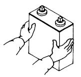
USE EDGE OF MODULE WHEN POSITIONING BATTERY
