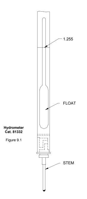
Periodically clean the hydrometer barrel and float with soap and water for ease of reading and improved accuracy.
