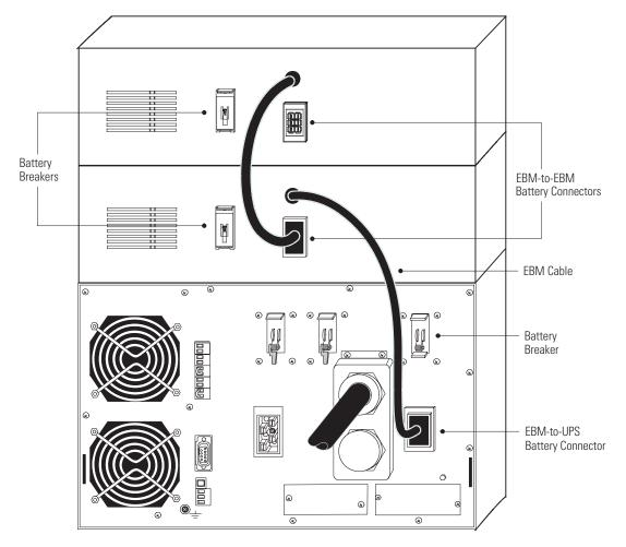
Figure 39. Typical EBM Installation
