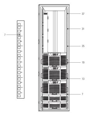
Recommended rail locations are for example only. Adjust the locations as needed for your system's configuration. Allow for hole spacing and numbering. For guidelines for configuring a parallel system with EBMs, see page 3.
