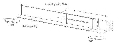
2. Select the proper holes in the rail for positioning the EBMs in the rack.
