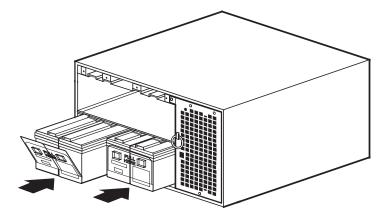
Figure 86. Installing the UPS Single-string Battery Trays for BladeUPS 5.0 kVA
