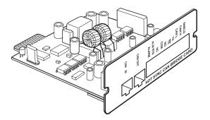
5. If there is a Jumper J7 on the Powerware Hot Sync CAN Bridge Card, remove and discard. See Figure 71.
