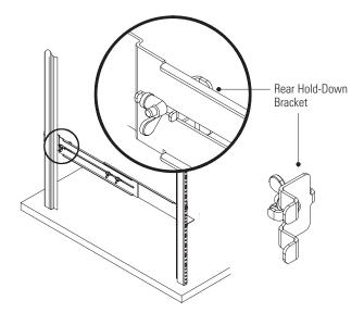
13. Verify that the brackets are seated firmly, then tighten the wing nuts on the rear hold-down brackets. The EBM is now secured in the rack.
