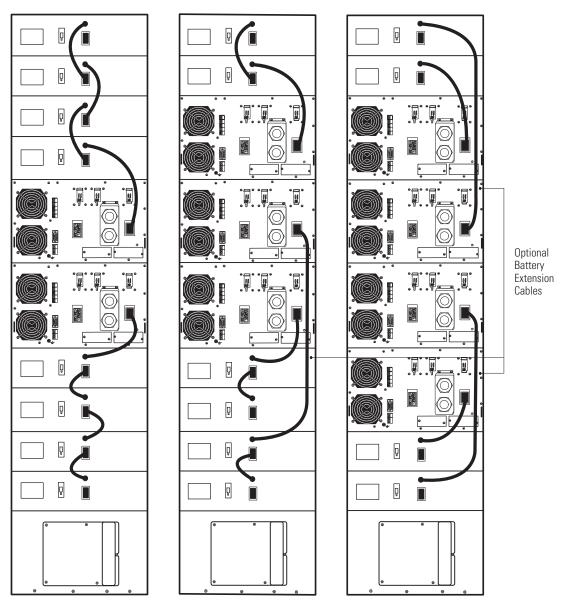
Figure 59. Example EBM Installations in Parallel Systems
