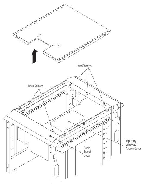
Remove the six screws on the conduit landing plate and retain. Remove and retain the plate (see <u>Figure 17</u>).
