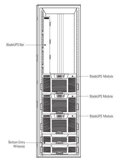
Figure 3. Example of a BladeUPS Parallel System
