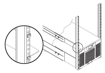
4. Using two clip nuts and two hex-head screws, attach the rail to the rear of the rack (see <u>Figure 34</u> and <u>Figure 35</u>).
