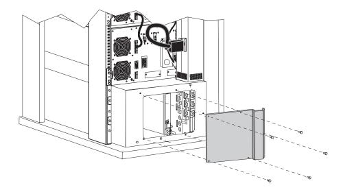
3. Remove the six screws on the conduit landing plate and retain. Remove the plate and retain. See Figure 22
