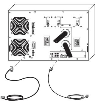
Connect the cables to the appropriate location. See <u>6.3 Communication Options</u> or <u>6.6 Control Terminals</u>for detailed information.
