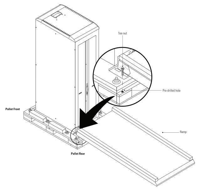
Figure 7. Attaching the Ramp to the Pallet
