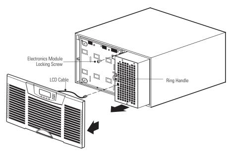
4. Label the original module with masking tape or some other identifier. Record the serial number of the replacement module for your warranty.
