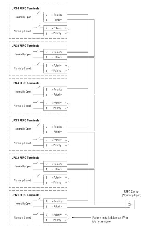
Figure 81. Normally-Open REPO Switch Wiring in a Parallel System
