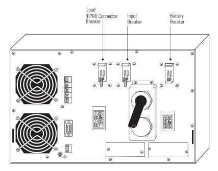
2. Remove the five screws on the bottom entry wireway access cover and retain. Remove the cover and retain (see Figure 21).
