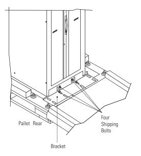
4. If the leveling feet are not fully retracted, turn the leveling feet clockwise until they are retracted (see Figure 9).
