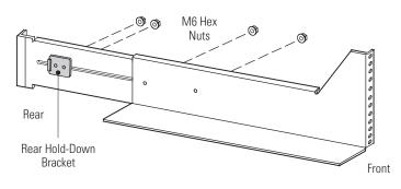
Verify that the holes in the rail align properly with the hole pattern in the rack. If the rack has square holes, verify that the studs on the end of the rail align within the square holes.
