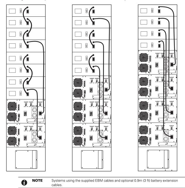
Figure 40. Example EBM Installations in Preassembled Parallel Systems
