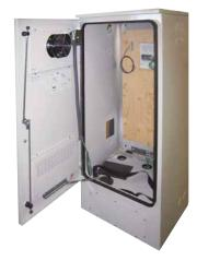
\*Install neoprene base gasket when pad mounting. \*\*Fan leads must be connected to power using the wire harness provided, 120 VAC, 10A breaker. \*\*\*All penetrations of the cabinet must utilize NEMA 3R rated components to maintain the cabinet rating.
