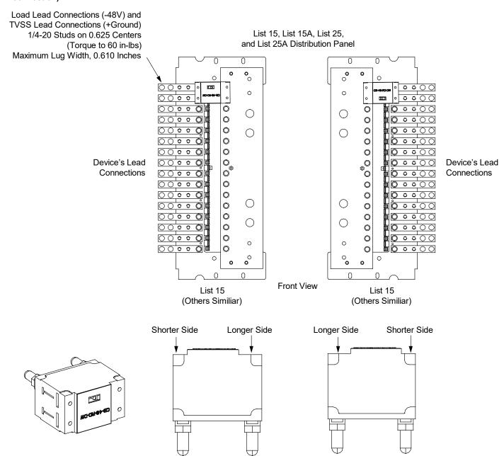
Install TVSS Device so Shorter Side is Towards the Device's Lead Connection Points
