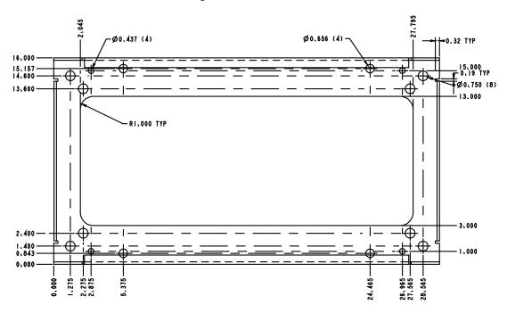
Figure 2: List 03 and List 09 Floor Hole Drilling Pattern Dimensions
