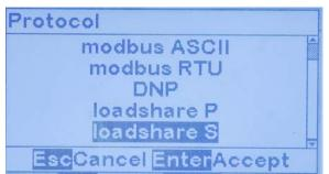
Select either "loadshare P" for the Primary ATevo, or "loadshare S" for a Secondary ATevo. Only one (1) ATevo can be the Primary. The other ATevo on the forced load sharing network must be set to Secondary.
