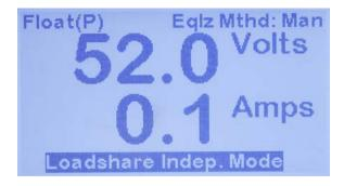
While in Virtual Independent mode, the ATevo will display the loadshare indicator and "Loadshare Indep. Mode" on the last line of the display.
