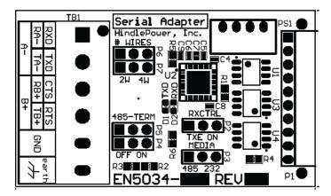
Jumper P2 (RXCNTRL) must be set to TXE - left two pins Jumper P3 (MEDIA) must be set to 485 - left two pins Jumpers P4 & P5 (485-TERM) must be set to OFF - left two pins Jumpers P6 & P7 (# WIRES) must be set to 2W - left two pins
