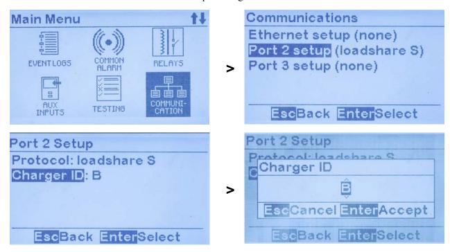
Use the UP and DOWN arrows to select the Charger ID (A, B C, or D). Each ATevo on the forced load sharing network must have a unique Charger ID (typically the Primary ATevo's Charger ID is set to 'A').
