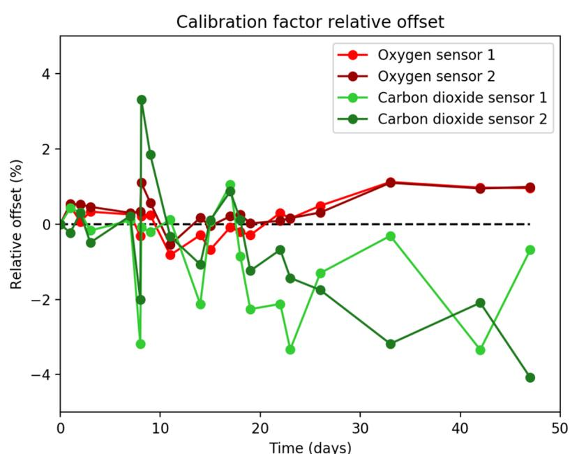
**Figure 1.** Relative drift of two O<sub>2</sub> and two CO<sub>2</sub> sensors over 40+ days while running continuously in active microbial fermentations.
