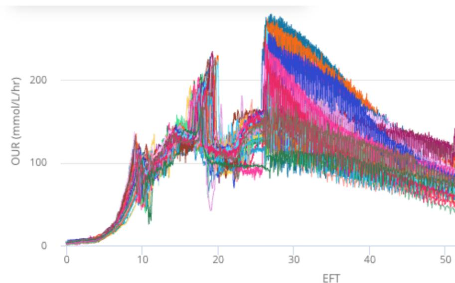
**Figure 5.** Oxygen uptake rate (OUR) from the 52 parallel bioreactor runs. This graph was auto-generated using live streaming data from Culture Bioscience's cloud-based online monitoring technology.
