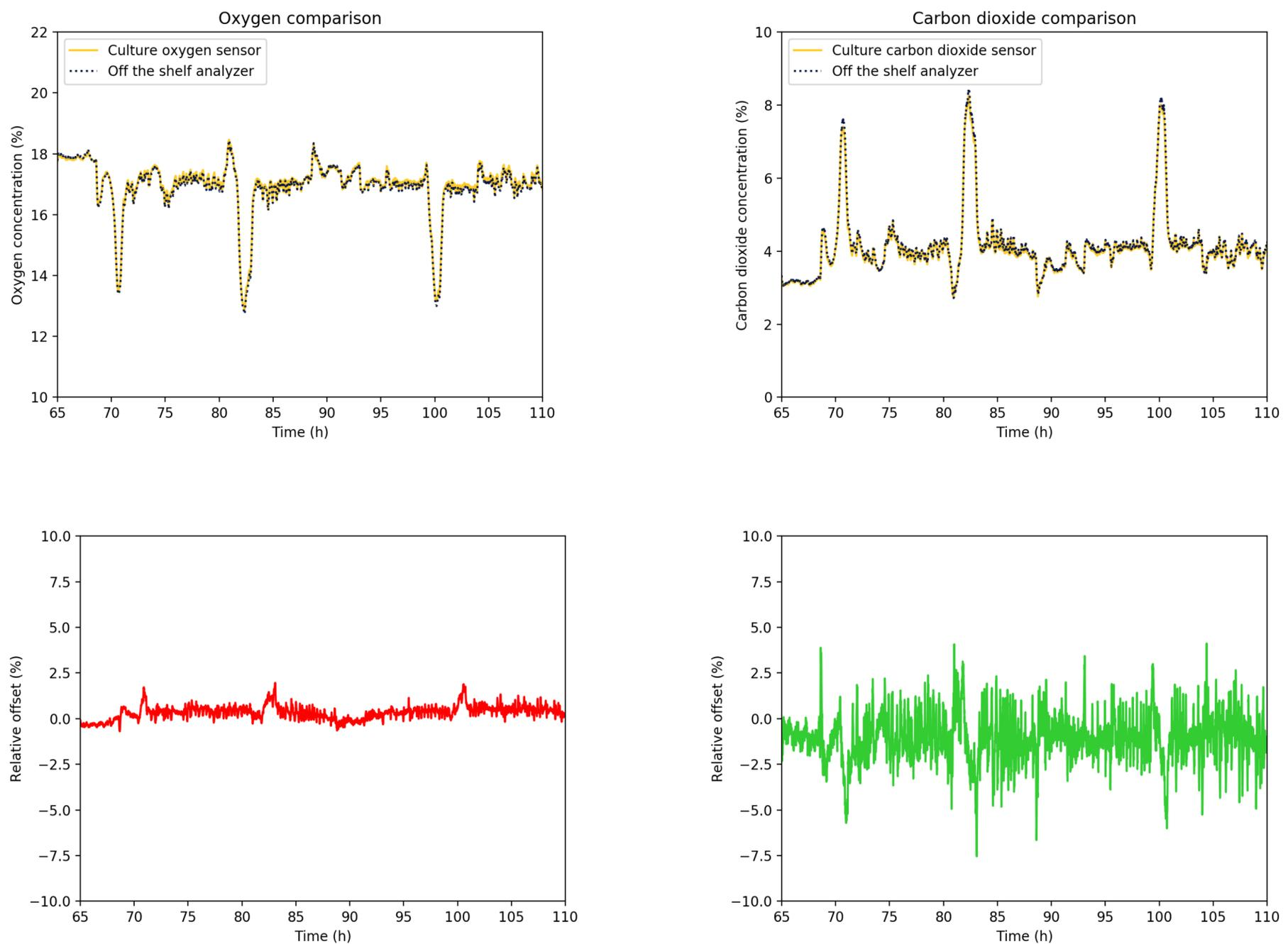
**Figure 3.** O<sub>2</sub> and CO<sub>2</sub> concentration of live yeast fermentations recorded by Culture Bioscience's off-gas analyzer and a commercially available off-gas analyzer. The relative percent offset from the Culture sensor and the off the shelf unit are plotted in the second row.
