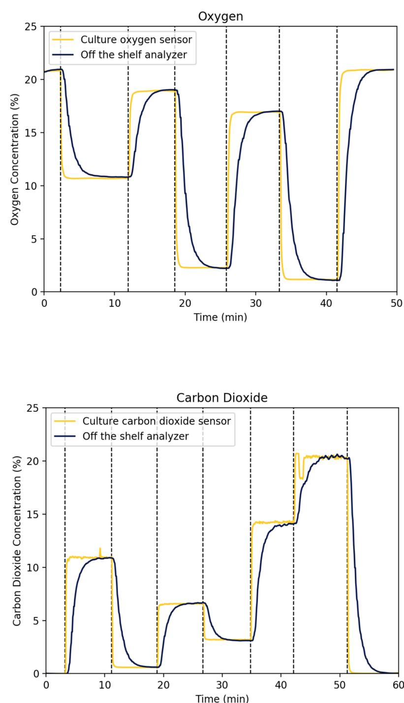
**Figure 2.** O<sub>2</sub> and CO<sub>2</sub> concentration of dry gas mixture step changes recorded by Culture Bioscience's off-gas analyzer (yellow) and a commercially available gas analyzer (blue). Step changes in gas concentration are marked with dashed vertical lines.
