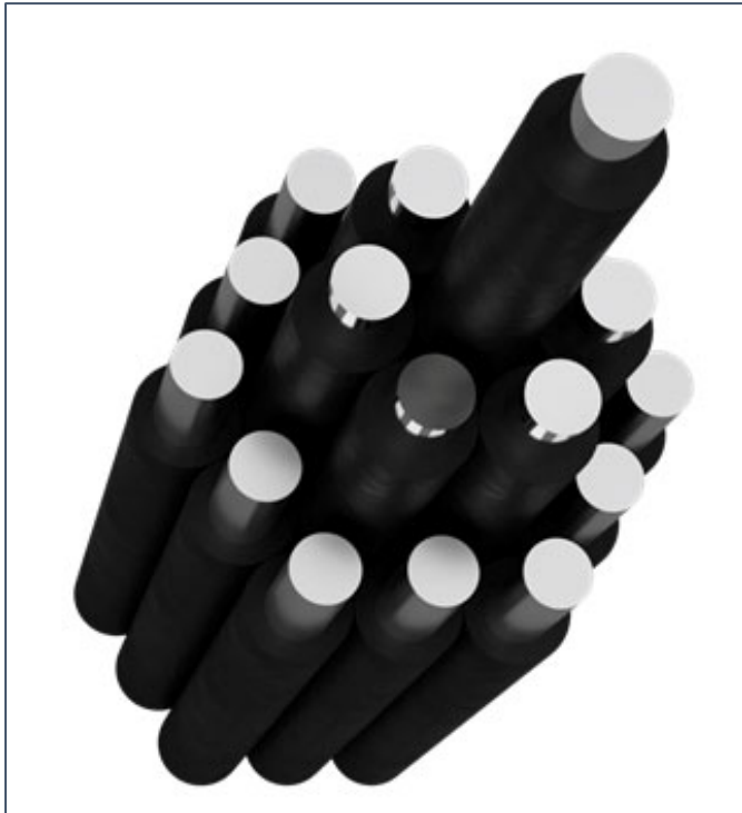
Figure 1 - Visualization of Cable Bundle (Conductors and Insulators)
